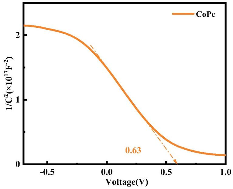
**Fig S10** The  $C-V$  characteristics of  $\text{Sb}_2(\text{S,Se})_3$  solar cell with CoPc HTLs
