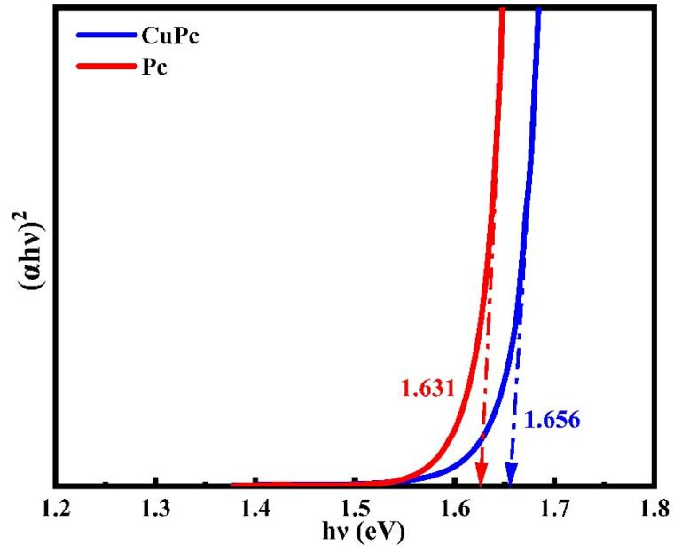
Fig S8 The band gap of CuPc and Pc hole transport layer
