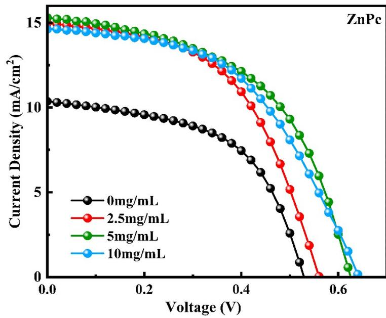
**Fig S4** The efficiency of  $\text{Sb}_2(\text{Se,S})_3$  solar cell with different concentration of ZnPc as hole transport layer
