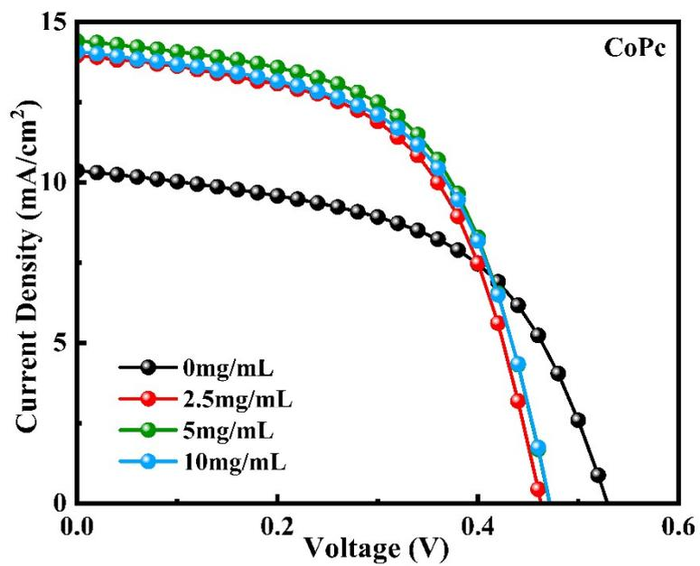
**Fig S2** The efficiency of  $\text{Sb}_2(\text{Se,S})_3$  solar cell with different concentration of CoPc as hole transport layer
