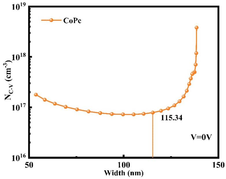
**Fig S11** The  $N_{C-V}$  characteristics of  $\text{Sb}_2(\text{S,Se})_3$  solar cell with CoPc HTLs
