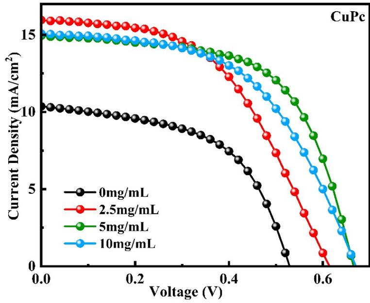
**Fig S3** The efficiency of  $\text{Sb}_2(\text{Se,S})_3$  solar cell with different concentration of CuPc as hole transport layer
