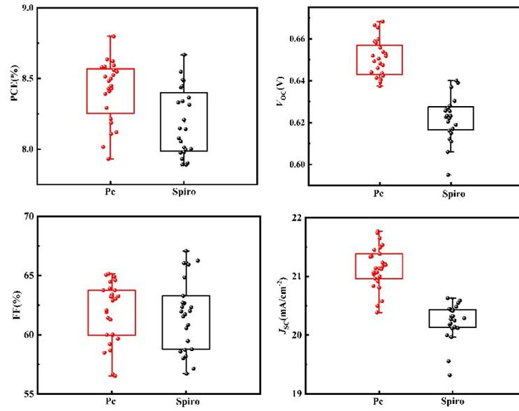
**Fig S9** The statistical deviation of the device with Pc and Spiro as the hole transport layer
