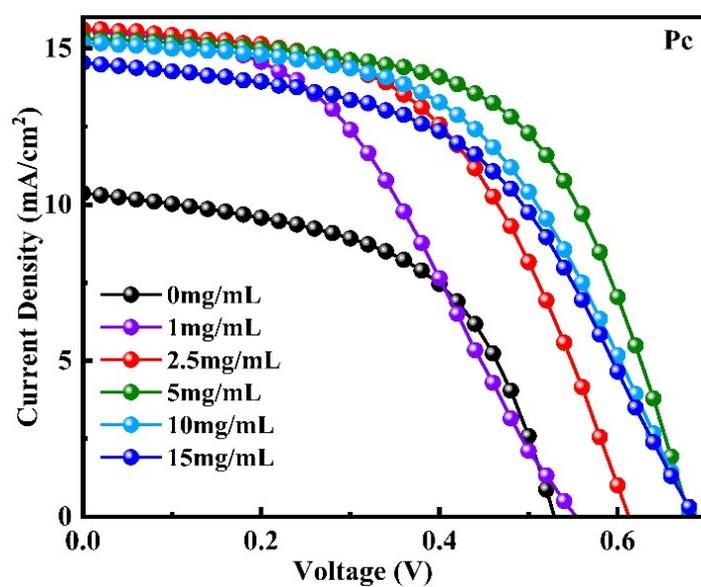
**Fig. S1** The efficiency of  $\text{Sb}_2(\text{S,Se})_3$  solar cells with various concentration of pure phthalocyanine as hole transport layer.
