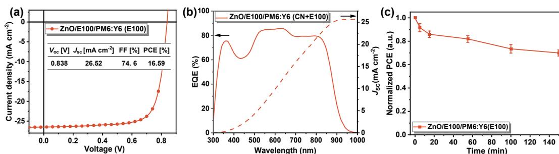
**Figure S8.** a)  $J$ - $V$  curve and the corresponding photovoltaic parameters and b) EQE spectrum. c) photostability plots under UV irradiation (365 nm, 50 mW cm<sup>-2</sup>) in ambient atmosphere of the PM6: Y6: E100-based i-OSCs with ZnO/E100 as ETL (error bars show standard deviation from the arithmetic mean value of 3 devices).
