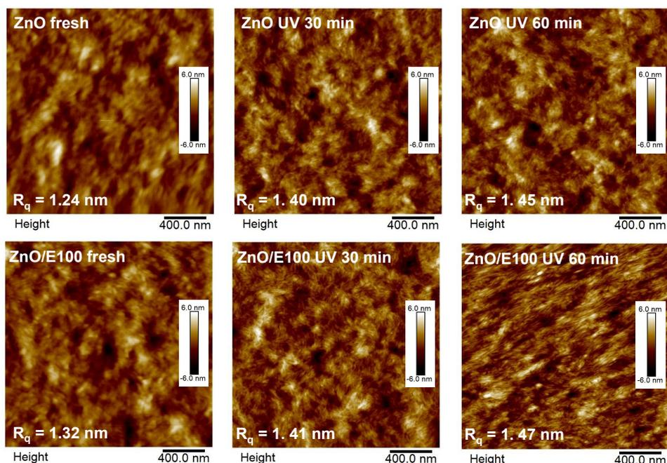
**Figure S7.** AFM topography images of chloroform processed PM6:Y6 (1:1.2, w/w) blend based on different ETLs before and after UV irradiation.
