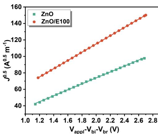
**Figure S1.**  $J^{0.5}$  vs ( $V_{app} - V_{bi} - V_{br}$ ) plots of electron only devices based on PM6:Y6 blend films with ZnO or ZnO/E100 as ETL.
