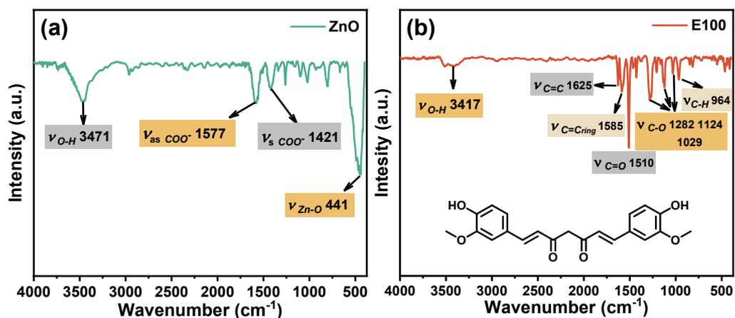
**Figure S2.** FT-IR spectra of (a) ZnO<sup>1</sup> and (b) E100<sup>2</sup> films.
