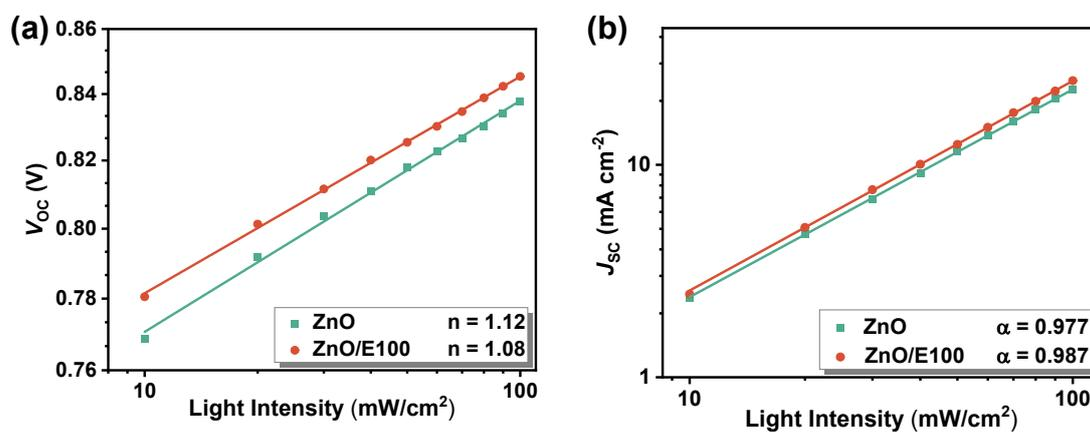
**Figure S6.** a)  $V_{oc}$  and b)  $J_{sc}$  versus light intensity plot based on PM6:Y6 blend films with ZnO or ZnO/E100 as ETL.
