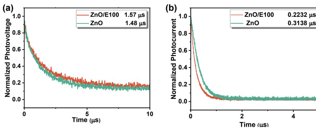
**Figure S5.** a) transient photovoltage and b) transient photocurrent profiles based on PM6:Y6 blend films with ZnO or ZnO/E100 as ETL.
