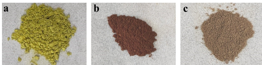
Figure S5. Photos of (a) Si NFs, (b) H-Si NFs, and (c) P-Si NFs.
