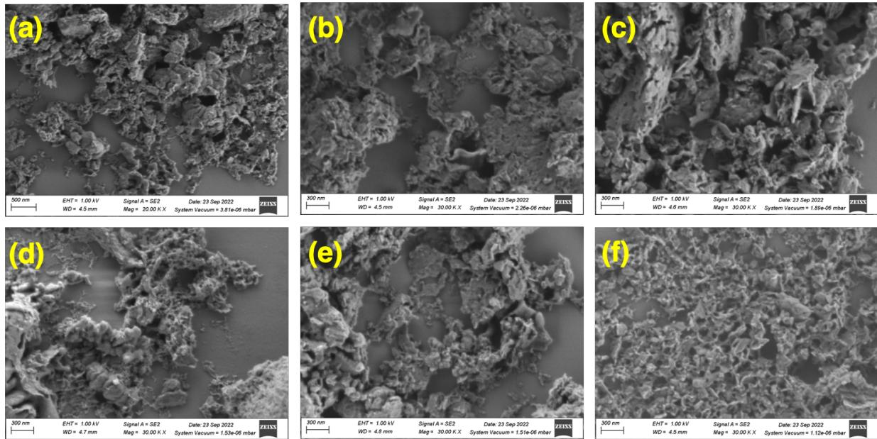
**Figure S2.** SEM images of the PgCN samples prepared using various methodologies (a) TP, (b) MP, (c), Stirr, (d) Probe, (e) SE, and (f) FD.
