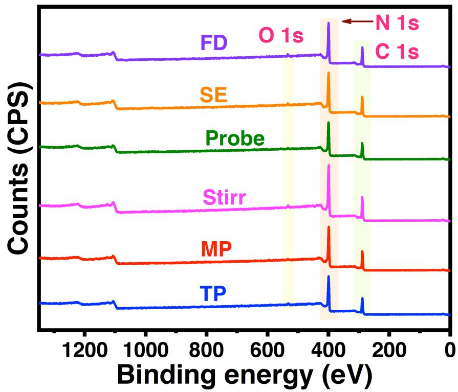
**Figure S3.** XPS survey spectra of various samples.
