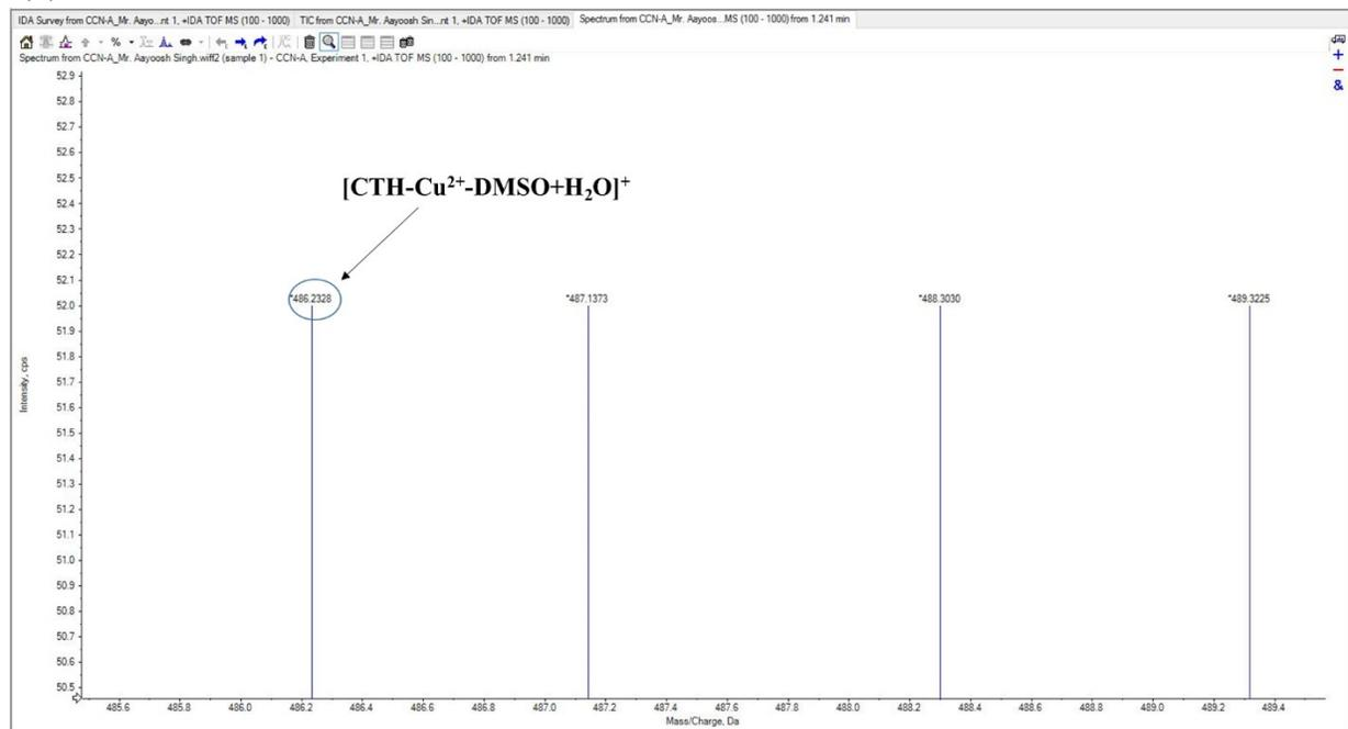
**Fig. S18 (a)** Mass spectrum of  $\text{CTH-Cu}^{2+}$  complex, **(b)** Molecular ion peak at  $m/z=486$ .
