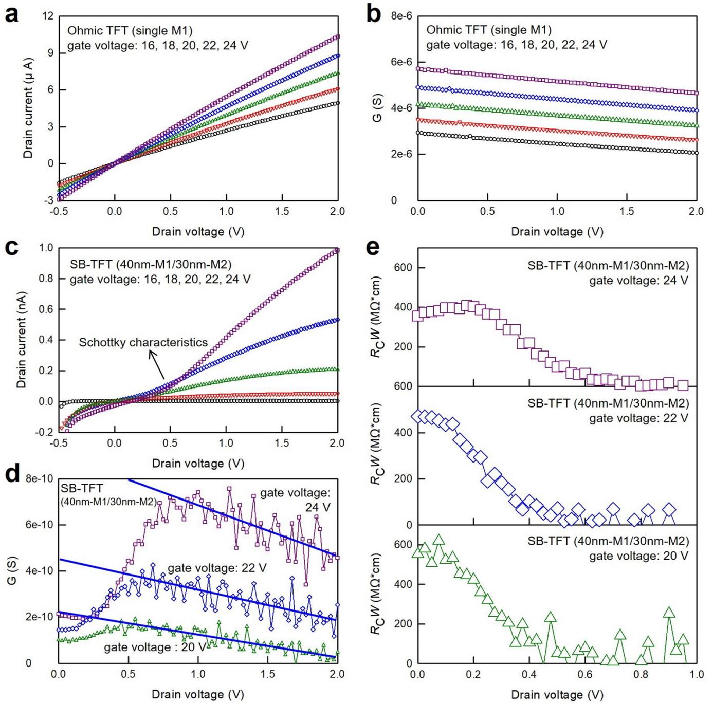
**Figure S8.** (a) The output characteristic curves and (b) output conductance of the ohmic TFT in a small- $V_D$  region. (c-e): The G-function analyses. (c) The output characteristic curves, (d) output conductance with linear fit lines, and (e) extracted  $R_C$  of the SB-TFT with the 40 nm-M1/30 nm-M2 SD electrodes in a small- $V_D$  region.
