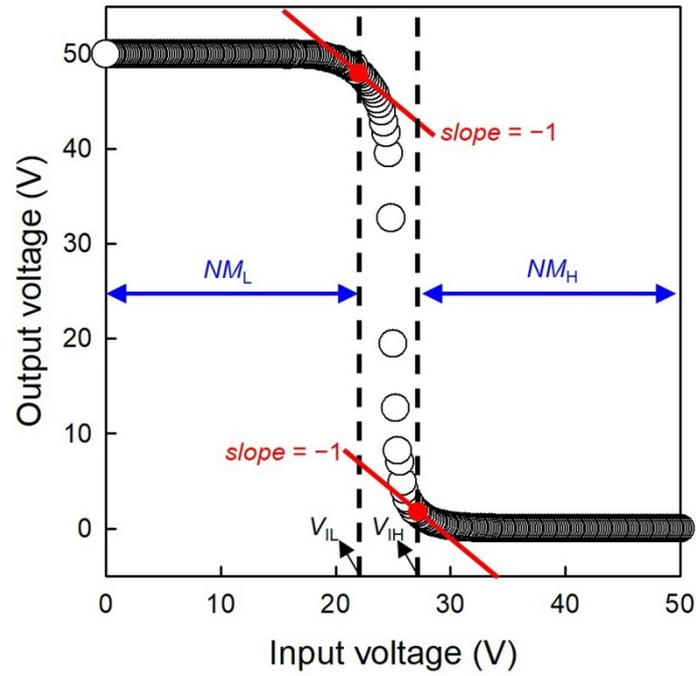
**Figure S11.** The details for the noise-margin calculation from the voltage transfer characteristic of the complementary inverter.
