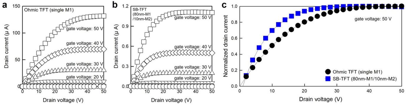
**Figure S7.** The output characteristic curves of (a) the ohmic TFT and (b) the SB-TFT with the 80 nm-M1/10 nm-M2 SD electrodes, respectively. (c) The normalized  $I_D$  vs.  $V_D$  plots of the IGZO SB-TFT and the IGZO ohmic TFT.
