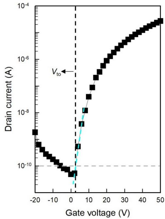
**Figure S2.** An example of the  $V_{to}$  extraction. The  $V_{to}$  extraction from the transfer characteristic curve of the IGZO SB-TFTs with the 80 nm-M1/10 nm-M2 SD electrodes.
