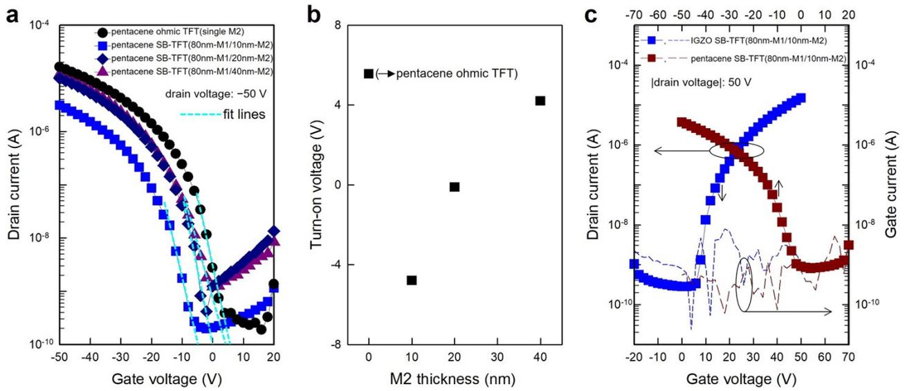
**Figure S10.** (a) The transfer characteristic curves of the pentacene SB-TFTs with the M1/M2 SD electrodes and the pentacene ohmic TFT, (b) the corresponding  $V_{to}$  values, and (c) the transfer characteristic curves (plotted together with the gate current) of the IGZO and pentacene SB-TFTs with the 80 nm-M1/10 nm-M2 SD electrodes.
