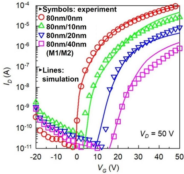
**Figure S9.** Comparison between the experimental and simulated transfer characteristics of the IGZO TFTs with the ohmic and M1/M2 SD contacts.
