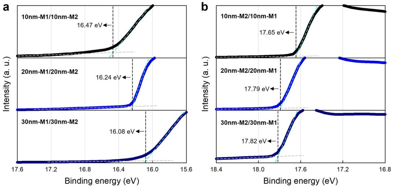
**Figure S5.** (a) The UPS spectra in the secondary-electron cut-off regions (with the corresponding fit lines and  $E_{co}$  values) in the M1/M2 case (i.e., 10 nm-M1/10 nm-M2, 20 nm-M1/20 nm-M2, and 30 nm-M1/30 nm-M2), and (b) those in the M2/M1 case (i.e., 10 nm-M2/10 nm-M1, 20 nm-M2/20 nm-M1, and 30 nm-M2/30 nm-M1).
