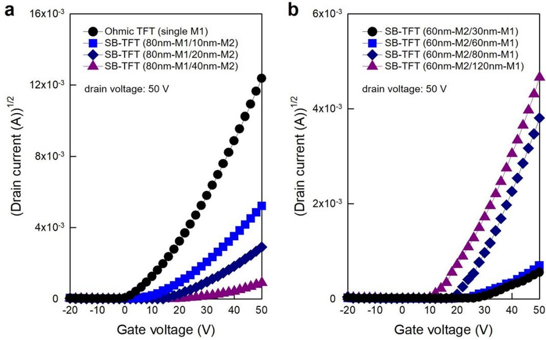
**Figure S3.** The  $I_D^{1/2}$  vs.  $V_G$  plots of (a) the IGZO SB-TFTs with the M1/M2 SD electrodes and the IGZO ohmic TFT and (b) those with the M2/M1 SD electrodes.
