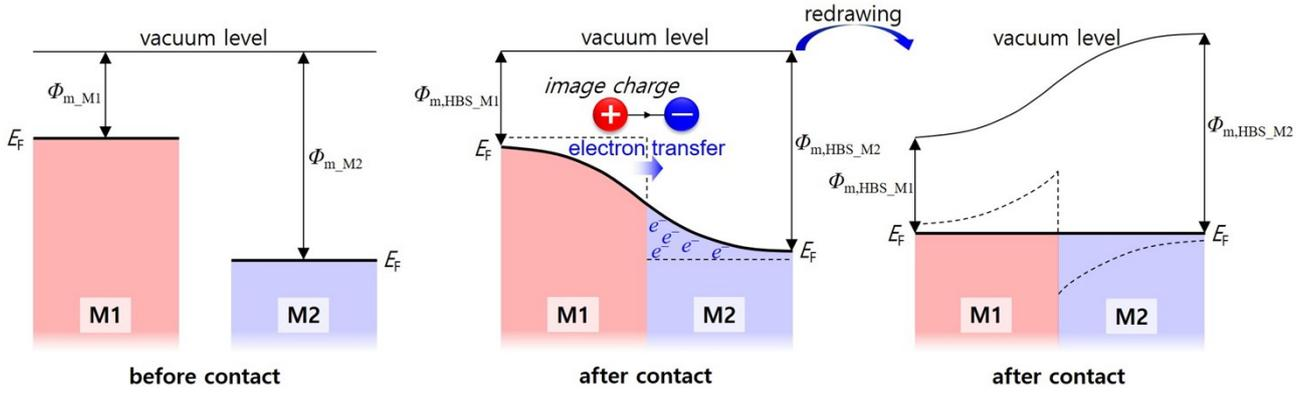
**Figure S1.** Schematic diagrams of the energy relations for the HBS-based thin film (i.e., with finite thickness).
