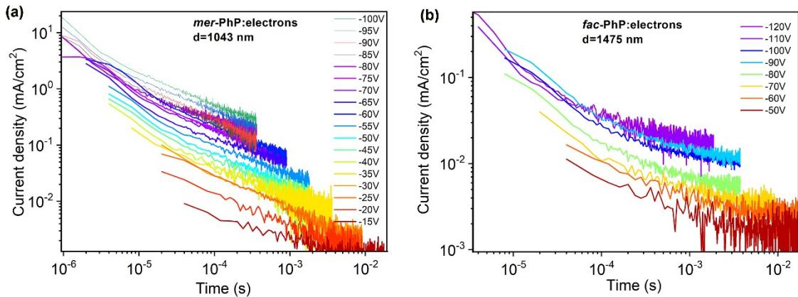
**Figure S6.** TOF transients for electrons for the layers of **mer-PhP** (a) and **fac-PhP** (b) recorded at the different voltages applied to ITO.  $t_{\text{tr}}$  were not observed.
