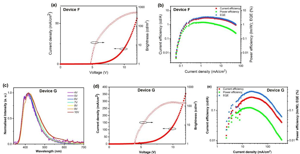
**Figure S11.** EL spectra at different voltages, dependencies of current density and brightness versus external voltage, current efficiency, power efficiency and EQE plots as the function of current density for *fac*-PhP based device F and G.
