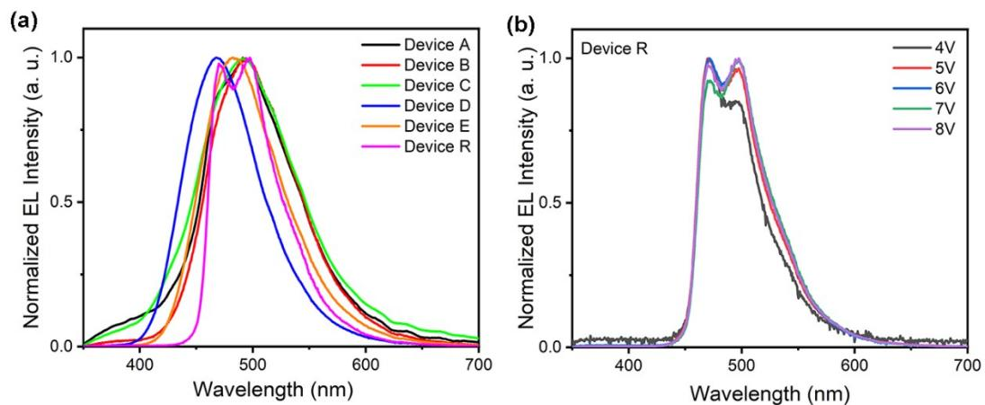
**Figure S9.** EL spectra of the devices A-E and R at 8 V (a). EL spectra of device R recorded at different driving voltages (b).
