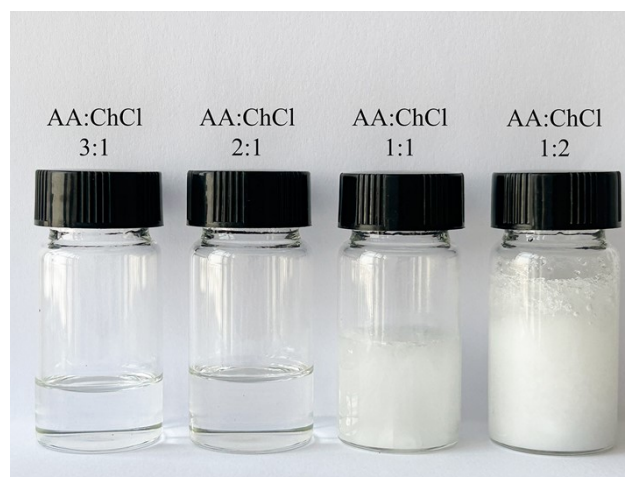
Figure S2. Digital images of PDES composed of different molar ratios (3:1 ~ 2:1) of AA: ChCl after cooling to room temperature.
