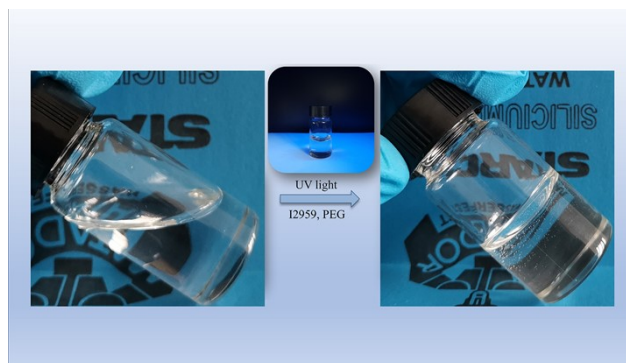
Figure S3. Comparative photos of PDES fluidity before and after polymerization.
