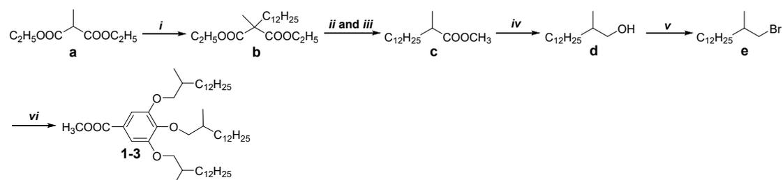
**Scheme S1.** Synthesis of the methyl 3,4,5-tris(dodecyloxy)benzoate with methyl branched chains (compound **1-3** in **Scheme S2**); Reagents and conditions: *i*)  $C_{12}H_{25}Br$ , NaH, THF, 0 to 75 °C; *ii*) KOH, EtOH, reflux; *iii*) a)  $N_2$ , 200 °C; b) *p*-toluenesulfonic acid, MeOH, reflux; *iv*)  $LiAlH_4$ , THF, 0 °C to RT; *v*) HBr,  $H_2SO_4$ (98%), tetrabutylammonium bromide, reflux; *vi*) methyl gallate,  $K_2CO_3$ , DMF,  $N_2$ , 90 °C.
