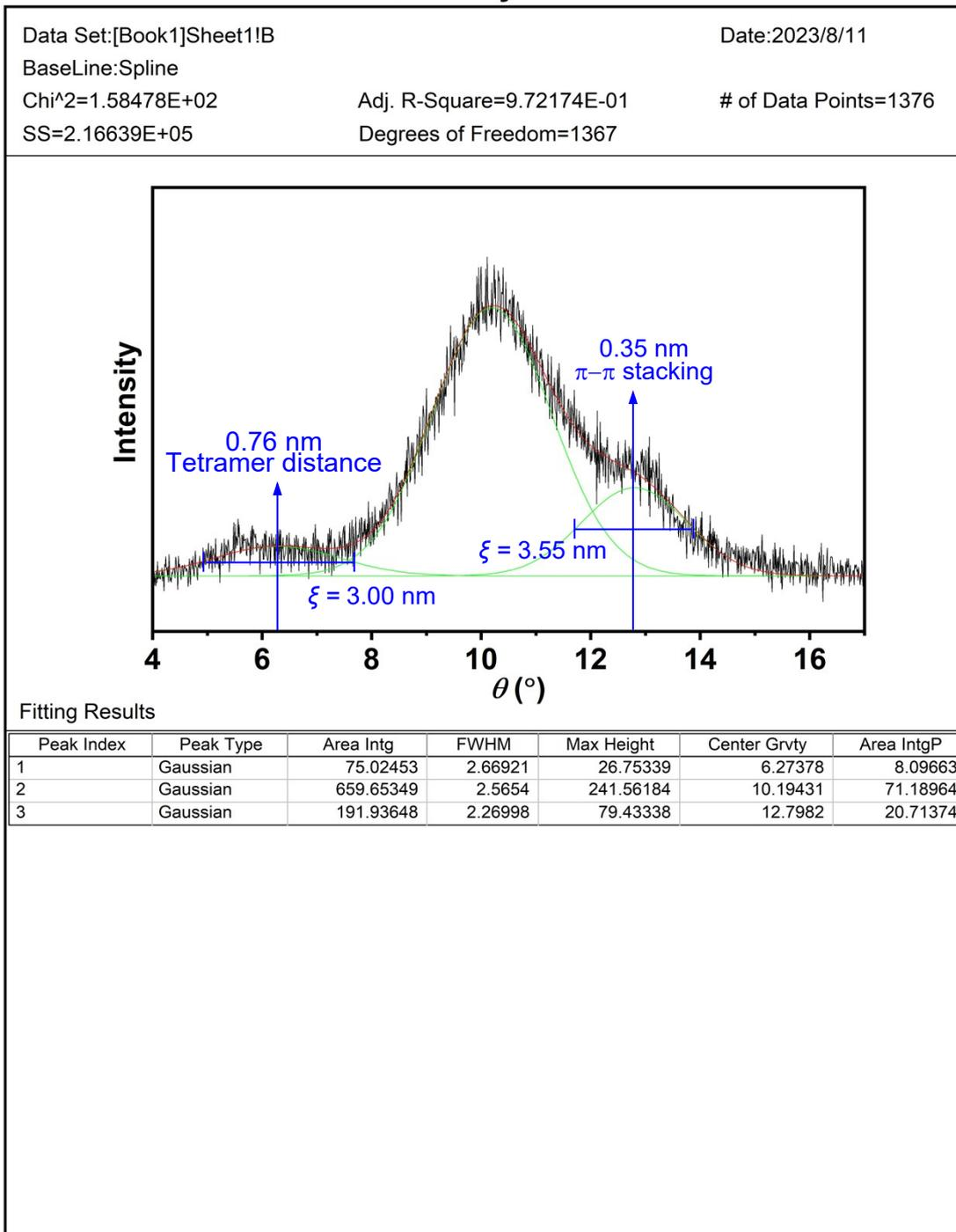
**Fig. S5** The representative diffraction plot at wide-angle region with peak deconvolution. The correlation length  $\xi$  is estimated from the full width at half-maximum (FWHM).
