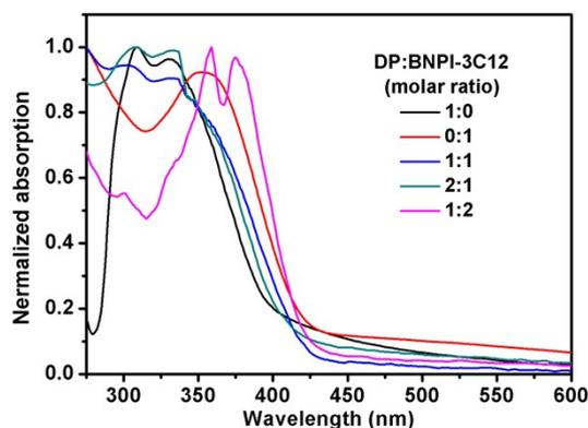
Fig. S9 UV-Vis absorption spectra BNPI-3C12/DP mixture in film.
