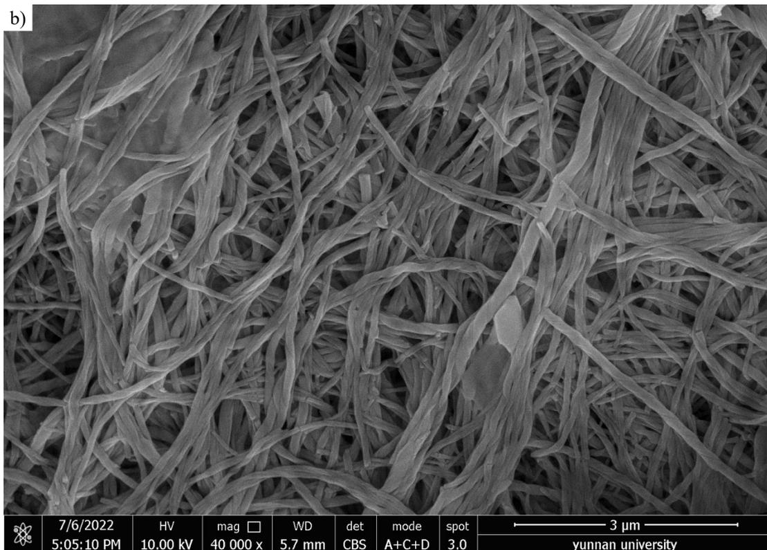
**Fig. S7** The large-scale SEM images with supramolecular nanohelix morphologies for the gels of a) **BNI-3C12** in DMF and b) **ABNI-3C12** in acetone, corresponding to that in Fig. 6.
