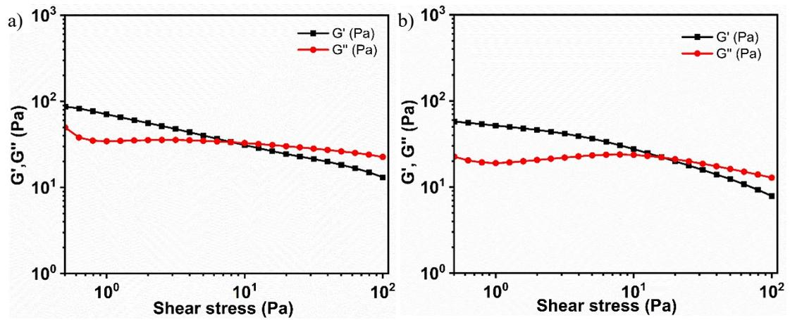
Fig. S6 Variation of storage modulus ( $G'$ ) and loss modulus ( $G''$ ) with shear stress
