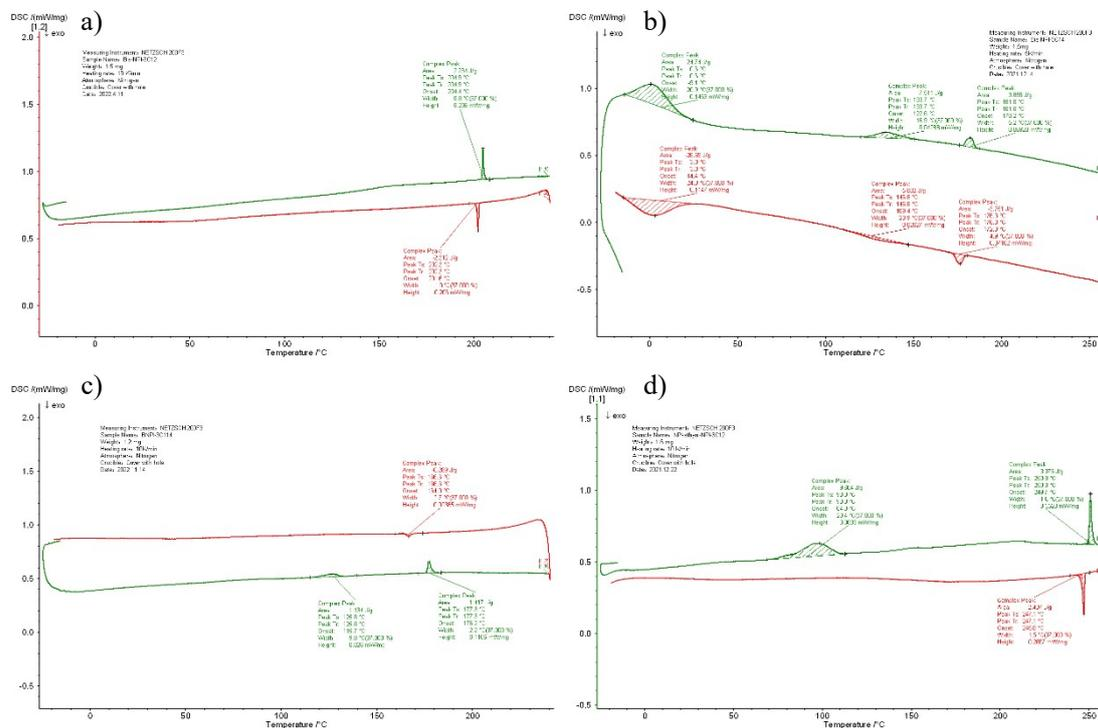
**Fig. S1** DSC curves of (a) compound **BNI-3C12** (10 K·min<sup>-1</sup>, first scan); (b) compound **BNI-3C14** (5 K·min<sup>-1</sup>, first scan); (c) compound **BNI-3C114** (10 K·min<sup>-1</sup>, first scan); compound **ABNI-3C12** (10 K·min<sup>-1</sup>, first scan).
