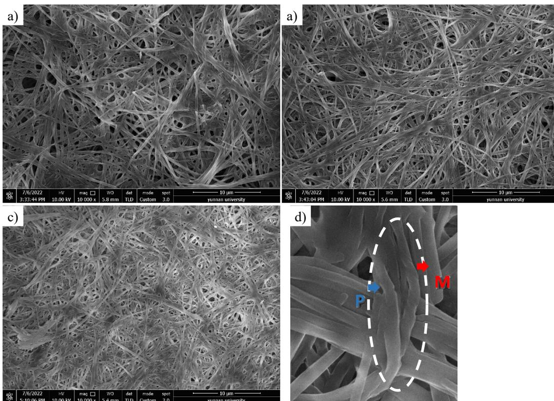
**Fig. S8** SEM images of the xerogel of **BNI-3C12** formed in a) ethyl acetate and b) n-butanol, and c) **ABNI-3C12** formed in DMF. Figure S6d is the partial enlarged detail of figure S6c with helical
