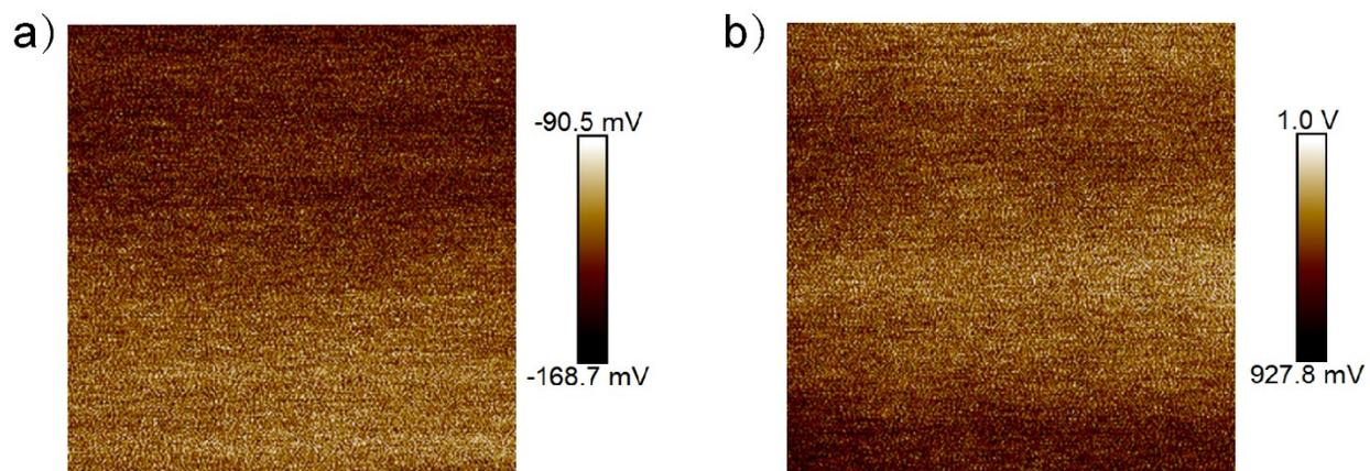
**Figure S3.** KPFM of MT-TP film before (a) and after (b) applying 1V bias through the probe.
