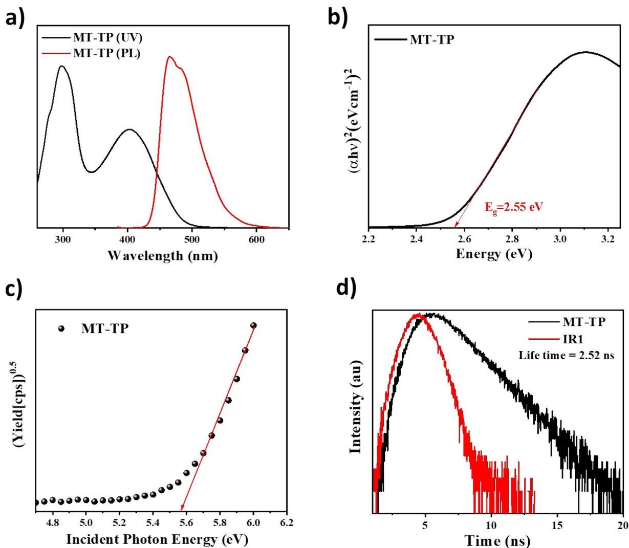
**Figure S2.** a) UV–visible absorption and b) photoluminescence spectra of MT-TP. c) Calculated HOMO of MT-TP COP by photoelectron spectroscopy (model: AC-2). d) Time-resolved PL spectra of MT-TP COP.
