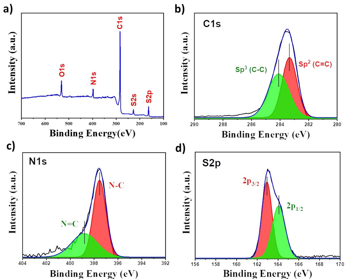
**Figure S1.** (a) XPS spectra and high-resolution spectra of (b) C 1s, (c) N 1s, and (d) S 2p peaks for MT-TP.
