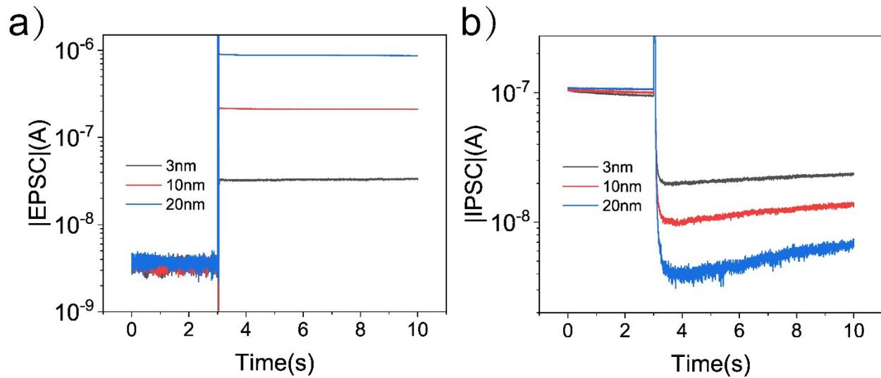
**Figure S4.** a)  $|EPSC|$  induced by positive gate pulse operation of different thickness of MT-TP (pulse amplitude: 50V, pulse width: 50 ms) with base  $V_{GS} = -5$  V and  $V_{DS} = -10$ V. b)  $|IPSC|$  induced by negative gate pulse operation of different thickness of MT-TP (pulse amplitude: -50V, pulse width: 50ms) with base  $V_{GS} = -5$ V and  $V_{DS} = -10$ V.
