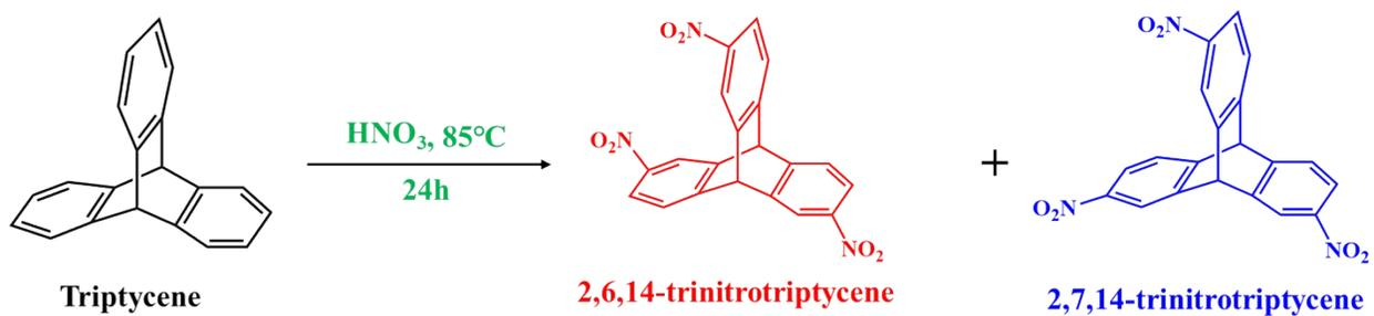
**Scheme S1.** Synthesis of Trinitrotriptycene.
