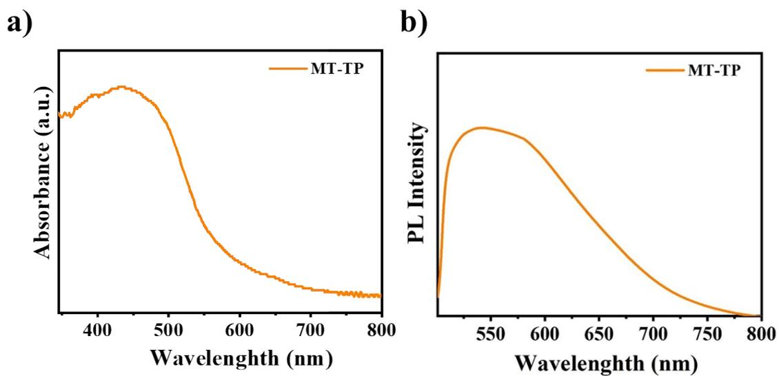
**Figure S6.** (a) UV-Vis and (b) PL emission spectra (at excitation wavelength of 400 nm) for MT-TP thin film.
