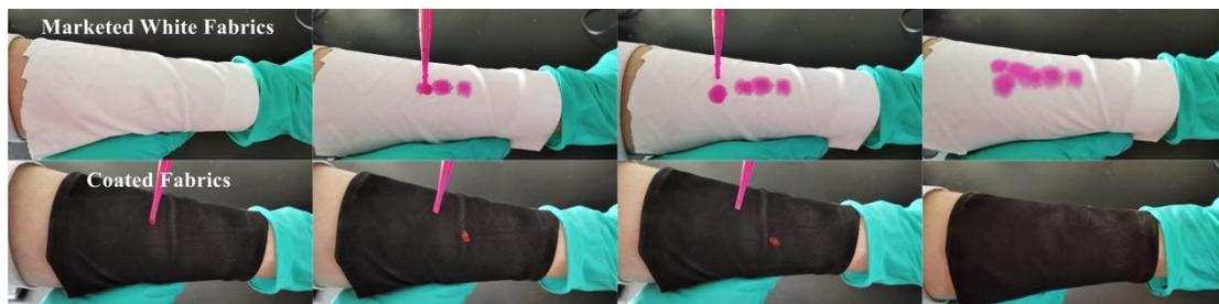
**Fig. S23.** Hydrophilicity of the original fabric and hydrophobicity of the coated fabric.
