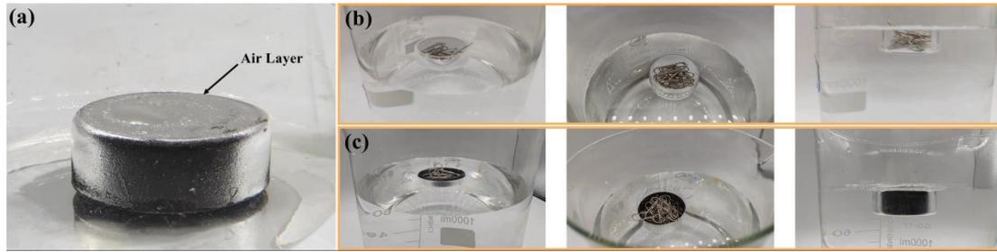
**Fig. S8.** (a) Silver mirror phenomenon in water for coated petri dishes; (b) Carrying capacity test for uncoated petri dishes; (c) Carrying capacity test for coated petri dishes.
