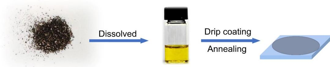
**Figure S3.** The schematic illustration of the preparation procedure of the  $\text{Cs}_4\text{CuSb}_2\text{Cl}_{12}$  thin film.
