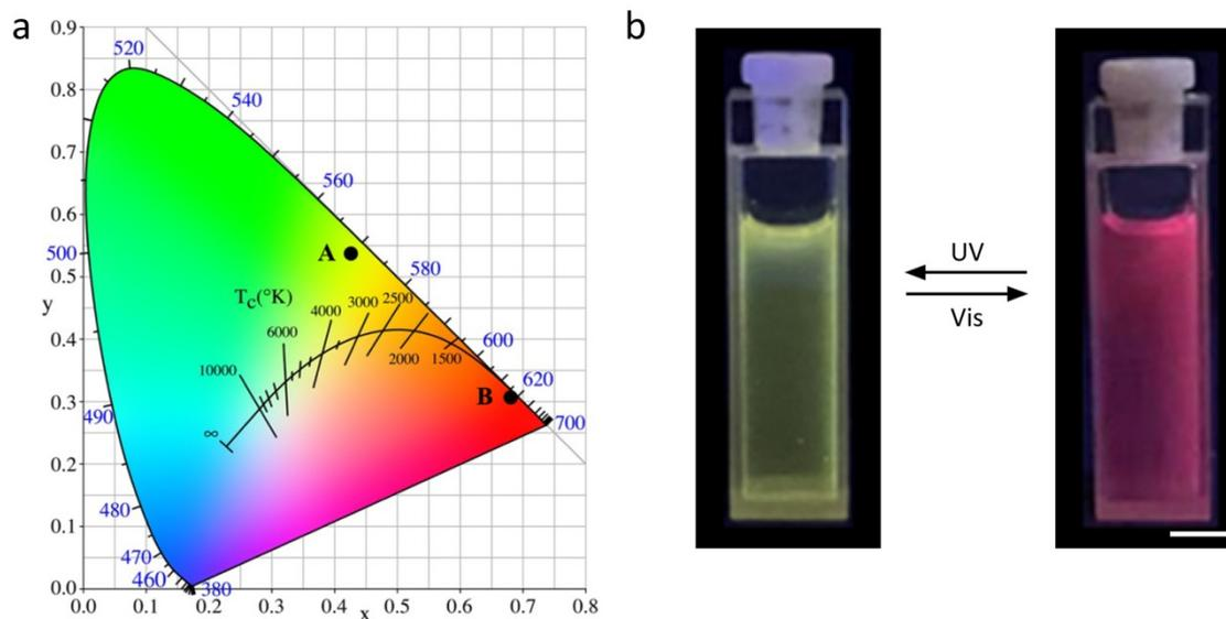
**Figure S14.** (a) CIE coordinates of supramolecular polymer solution SPS-4: A (initial state), B (after 365 nm UV irradiation). (b) Fluorescence transition of SPS-4. All scale bars are 0.5 cm.
