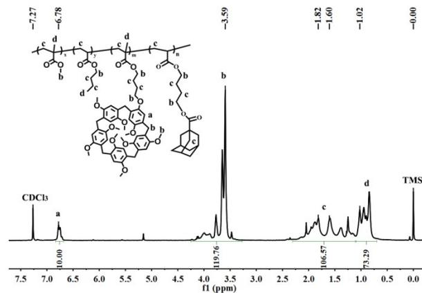
**Figure S10.**  $^1\text{H-NMR}$  spectrum (in  $\text{CDCl}_3$ ) of P(MMA-*co*-BA-*co*-P5A-*co*-AD).
