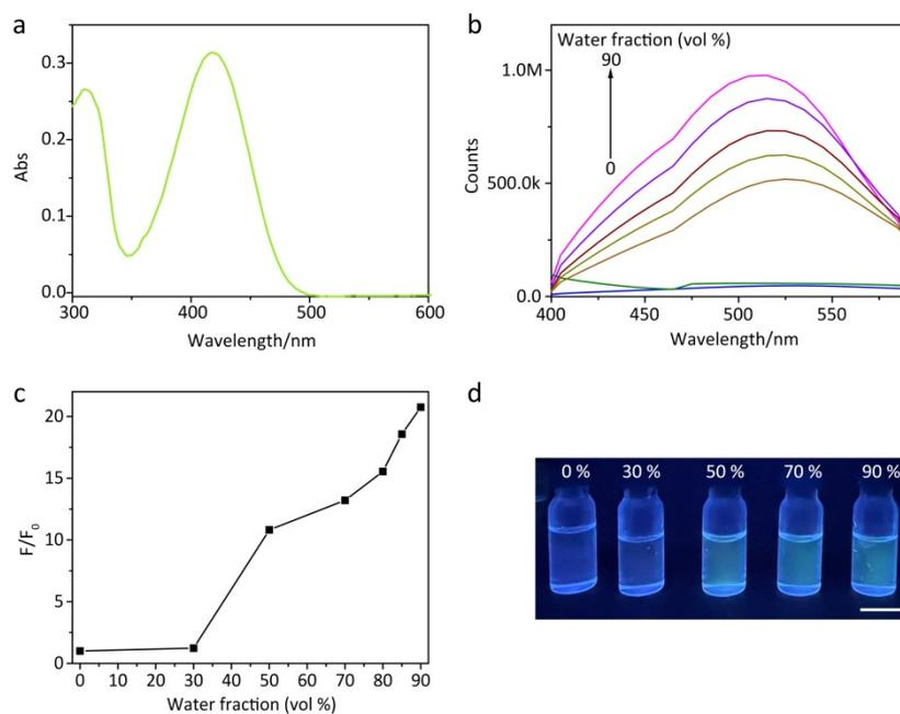
**Figure S7.** (a) The absorption spectra of NC-DSA-CN in DMSO. (b) Fluorescence emission spectra of NC-DSA-CN (10  $\mu\text{M}$ ) in water/DMSO mixtures,  $f_w = 0-90$  vol%. (c) Plot of peak intensity of NC-DSA-CN versus  $f_w$  in the mixtures. (d) The photographs of NC-DSA-CN (10  $\mu\text{M}$ ) in water/DMSO mixtures,  $f_w = 0-90$  vol%. The scale bars is 0.5 cm.
