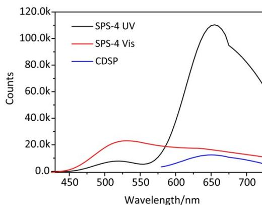
**Figure S13.** Fluorescence spectra of SPS-4 under alternating 365 nm UV and 525 nm Visible light (red trace:  $\lambda_{ex} = 365$  nm, black trace:  $\lambda_{ex} = 365$  nm, blue trace,  $\lambda_{ex} = 560$  nm). The blue trace represents the fluorescence spectrum ( $\lambda_{ex}=560$  nm) of CDSP in DMSO (1.8  $\mu\text{g/mL}$ ).
