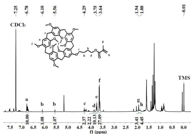
**Figure S2.**  $^1\text{H-NMR}$  spectrum (in  $\text{CDCl}_3$ ) of P5A-Aly.
