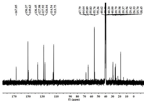
**Figure S3.**  $^{13}\text{C-NMR}$  spectrum (in  $\text{CDCl}_3$ ) of P5A-Aly.
