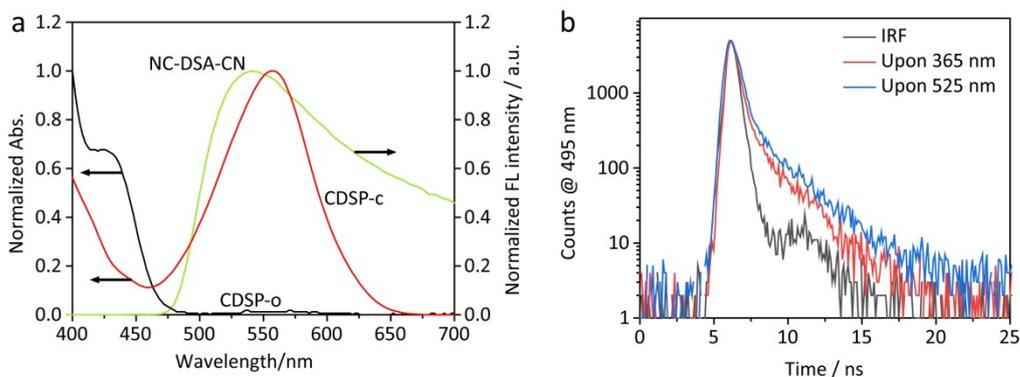
**Figure S12.** The normalized emission spectrum of NC-DSA-CN and the absorption spectrum of CDSP (before and after 365 nm UV irradiation) in DMSO. (b) Fluorescence lifetime changes of SPS-4 under alternating 365 nm UV and 525 nm Visible light.
