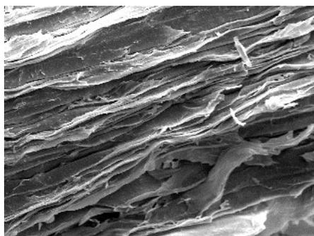
**Figure S1.** Cross-section SEM micrograph of rBC/MXene hydrogel after elongation break.
