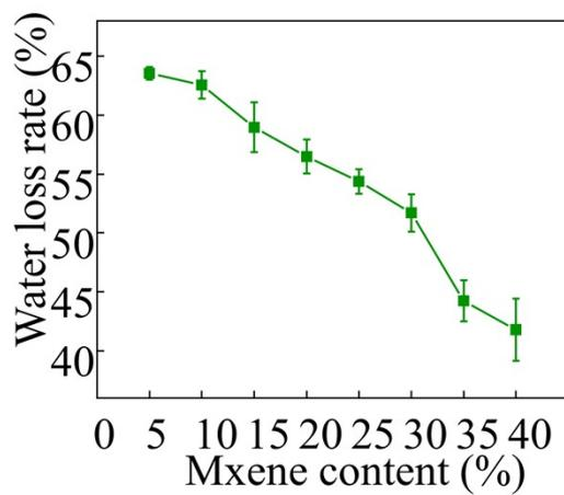
**Figure S4.** Water loss rate of hydrogels after stretching 100%.
