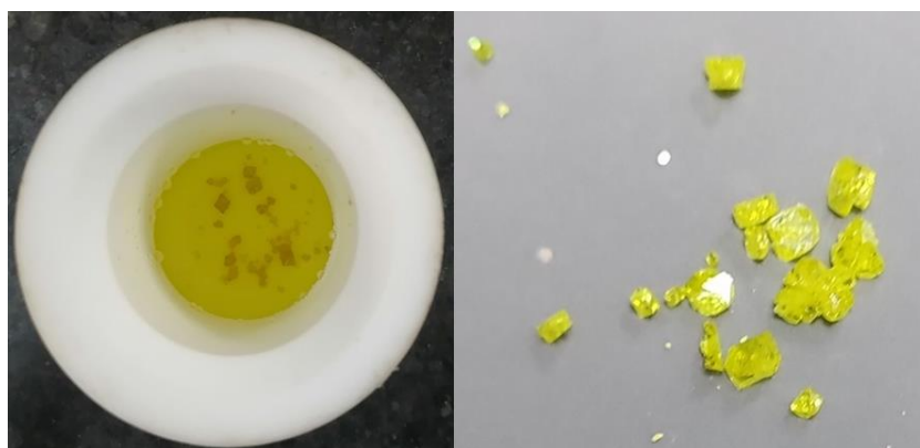
Image S1: Synthesized crystals of pristine \text{Cs}_2\text{AgBiCl}_6 (HT-0) DP.
