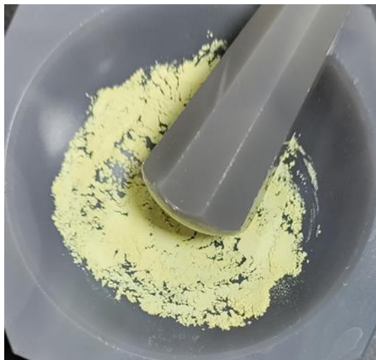
Image S4: Synthesis of Pristine \text{Cs}_2\text{AgBiCl}_6 (MCS-0).
