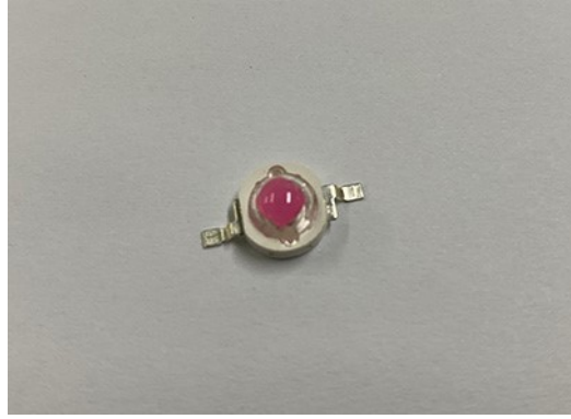
Figure S10. A photograph of an LED fabricated by ZIF-8@pm567A/SRh101 with a 460 nm blue LED chip.
