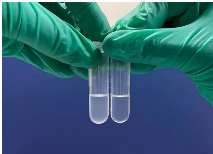
Figure S3. Optical appearance of the ILs dispersion by using pure THF as solvent (left) and using THF/DMF as solvent (right).
