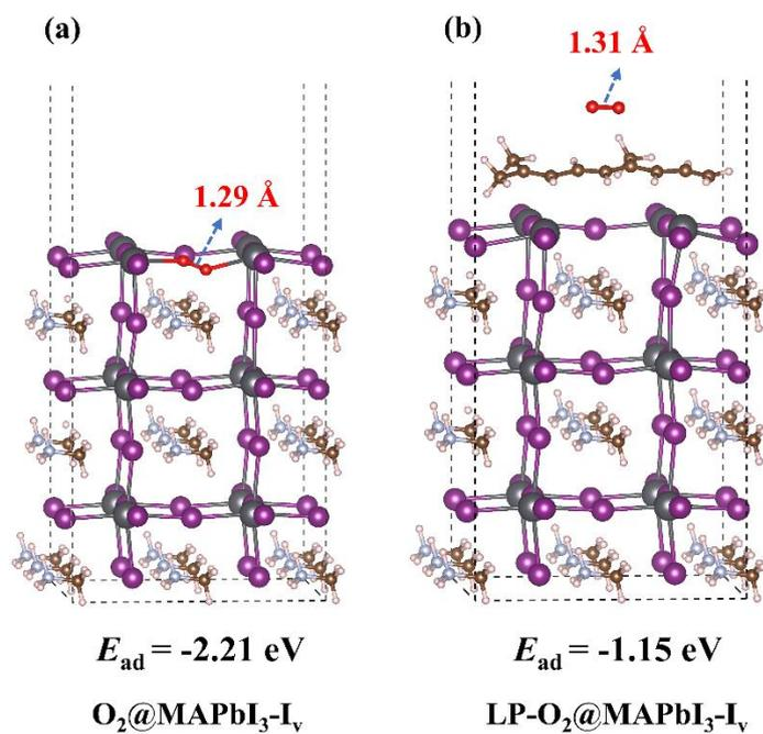
Figure S4. The side and top views of optimized configurations for (a)  $\text{O}_2@MAPbI_3-I_v$  and (b)  $LP-O_2@MAPbI_3-I_v$ .
