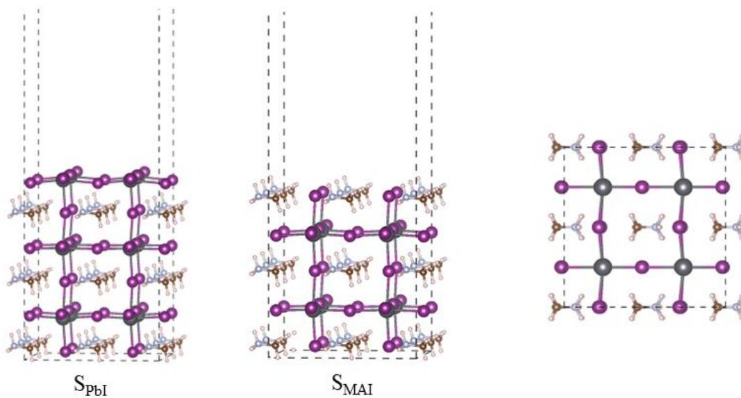
Figure S1. Side and top views of slab models of  $\text{PbI}_2$ -terminated ( $S_{\text{PbI}}$ ) and MAI-terminated ( $S_{\text{MAI}}$ ) (001) surfaces of  $\text{MAPbI}_3$ .
