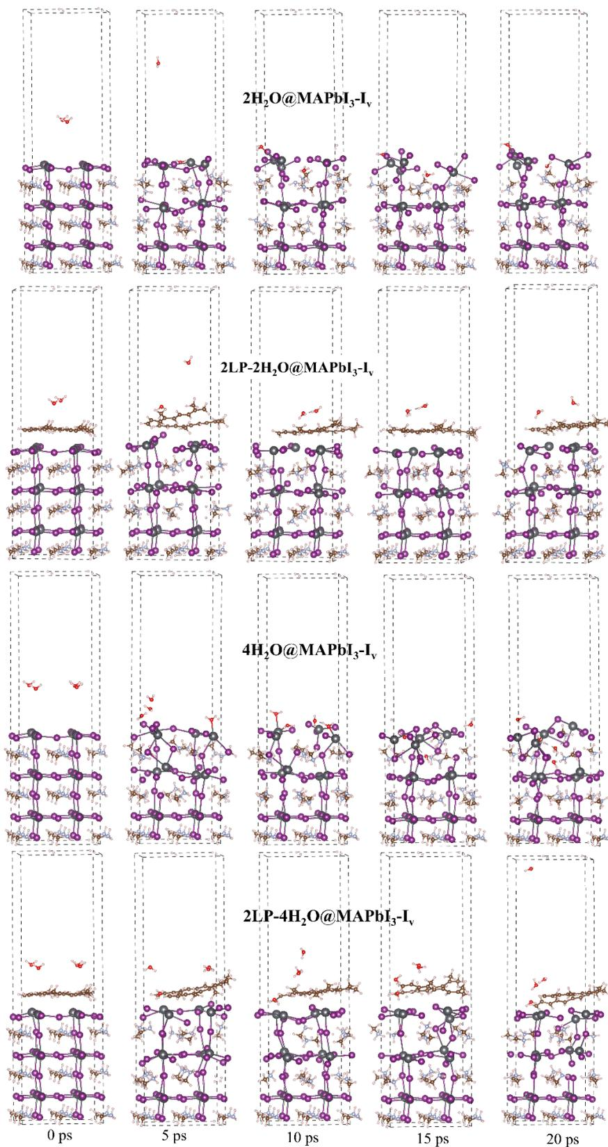
Figure S6. Snapshots of AIMD simulations at 0, 5, 10, 15, and 20 ps for 2H<sub>2</sub>O@MAPbI<sub>3</sub>-I<sub>v</sub>, 2LP-2H<sub>2</sub>O@MAPbI<sub>3</sub>-I<sub>v</sub>, 4H<sub>2</sub>O@MAPbI<sub>3</sub>-I<sub>v</sub>, and 2LP-4H<sub>2</sub>O@MAPbI<sub>3</sub>-I<sub>v</sub>.
