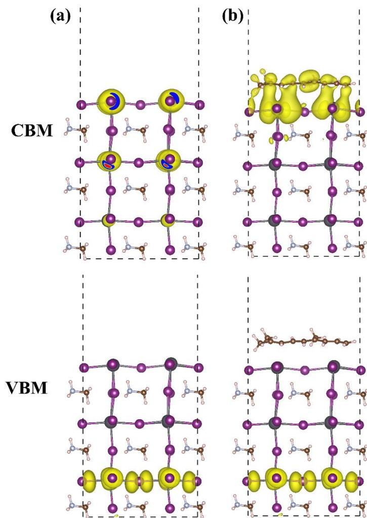
Figure S3. Charge densities of CBM and VBM for (a) MAPbI<sub>3</sub>-I<sub>v</sub> and (b) LP@MAPbI<sub>3</sub>-I<sub>v</sub>. The isosurface level is 0.0008 e/Bohr<sup>3</sup>.
