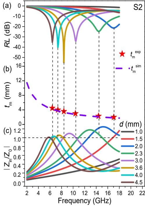
**Fig. S2** (a) Frequency-dependent  $RL$ , (b) simulation of  $t_m \sim f_m$  under the  $\lambda/4$  model and (c)  $|Z_{\text{in}}/Z_0|$  versus  $f$  curves of S2.
