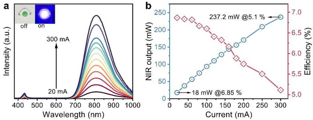
**Figure S4.** (a) Electroluminescence spectra of NIR I emission pc-LED (LED 2) driving by varied current, the insets show photographs of the LED 2 on and off. (b) The NIR output and photoelectric conversion efficiency of NIR I emission pc-LED (LED 2).
