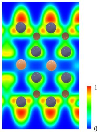
Fig. S2. Electron localization function of monolayer VC<sub>2</sub>N<sub>4</sub>.
