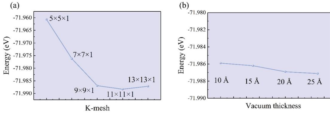
Fig. S1. The convergence tests of (a) K-mesh and (b) vacuum thickness.
