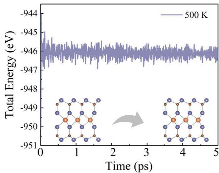
Fig. S3. Evolution of the total energy during 5 ps from AIMD simulation at 500 K; insets show the snapshots of initial and final structures of monolayer VC<sub>2</sub>N<sub>4</sub>.
