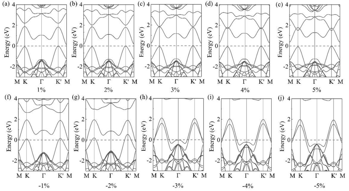
Fig. S6. Band structures of monolayer  $\text{VC}_2\text{N}_4$  with SOC under different strains.
