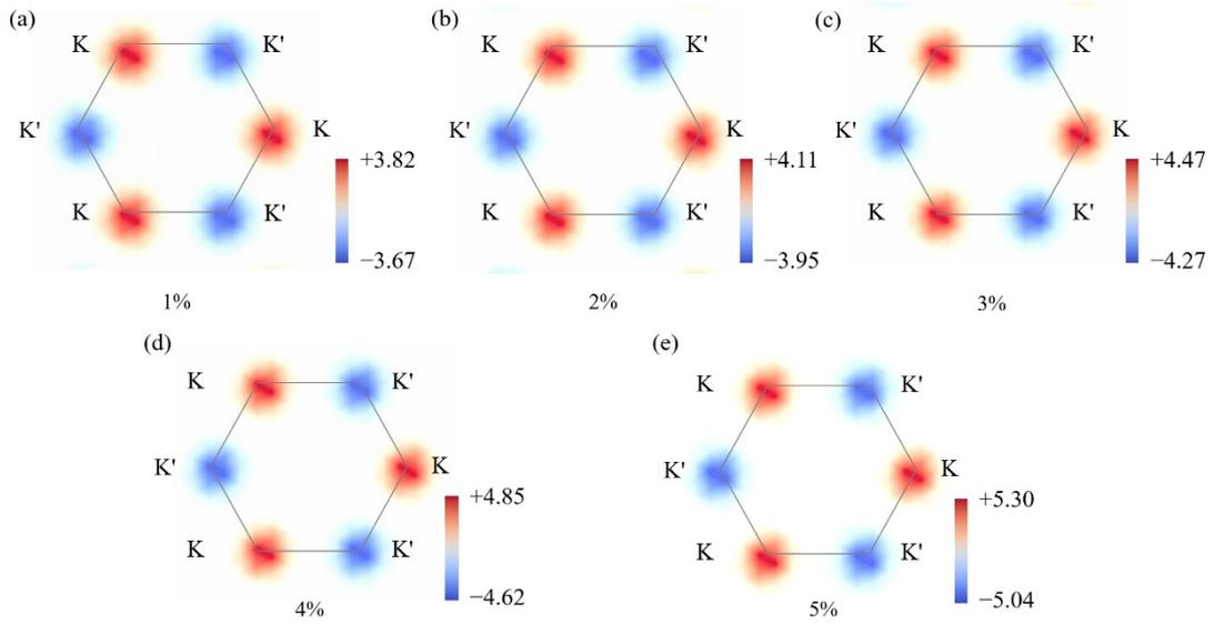
Fig. S7. Berry curvature of VB as a contour map over the 2D BZ for monolayer  $\text{VC}_2\text{N}_4$  under different strains.
