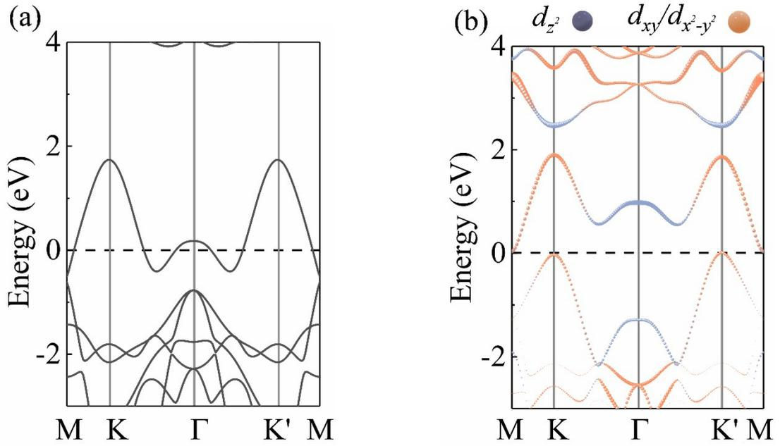
Fig. S4. (a) Band structure of monolayer VC<sub>2</sub>N<sub>4</sub> without spin polarization and SOC. (b) Orbital-resolved band structures of monolayer VC<sub>2</sub>N<sub>4</sub> with spin polarization and SOC.
