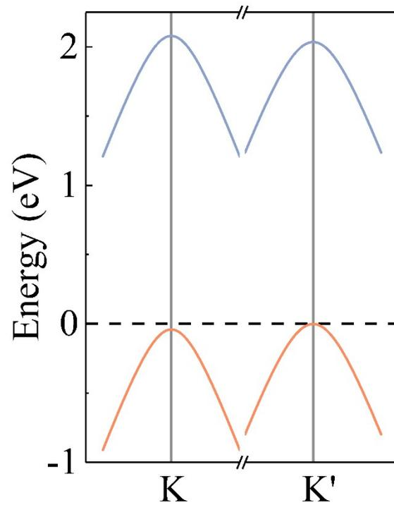
Fig. S5. Low-energy electronic bands around K and K' valleys based on the tight-binding models. The orange and blue lines are spin-up and spin-down states, respectively.
