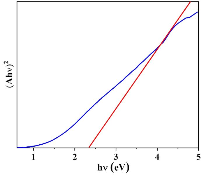
**Fig. S1** Tauc plot converted from the absorbance of VP nanoflakes.
