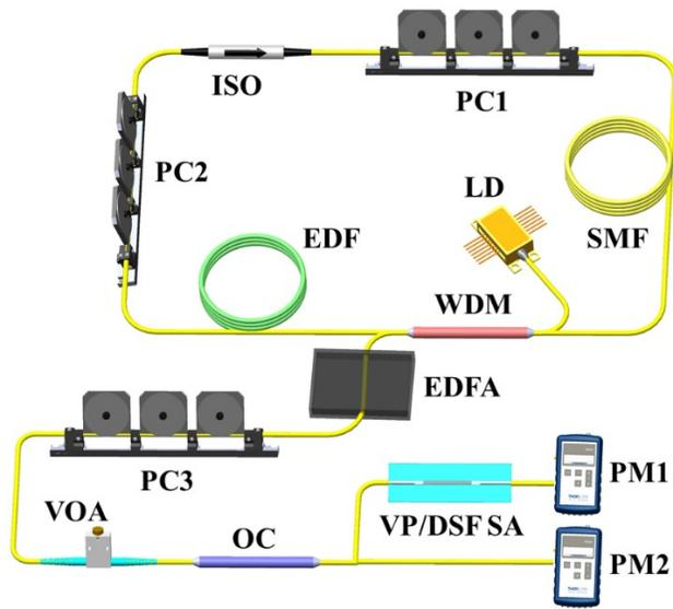
**Fig. S2** The balanced twin-detector fiber setup.
