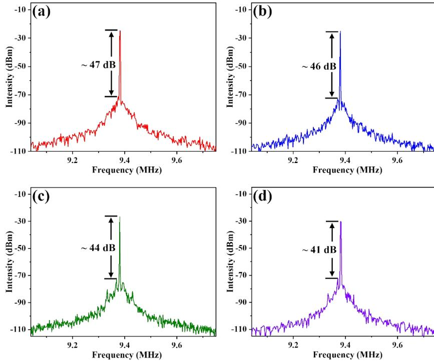
**Fig. S3** The SNRs of (a) the tightly bound two-pulse soliton molecule, (b) the loosely bound two-pulse soliton molecule, (c) the three-pulse bound soliton molecule, and (d) the four-pulse bound soliton molecule.
