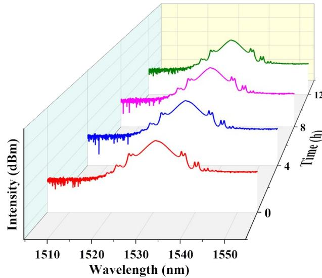
**Fig. S4** Optical spectra of mode-locked laser pulses recorded every 4 hours.
