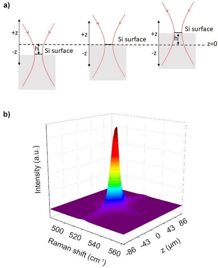
**Figure S2.** Schematic illustrating how a specific plane of illuminated bulk material (Si wafer) contributes to  $I_{bulk}$ , demonstrating the method for determining the depth dependency of the Raman signal.
