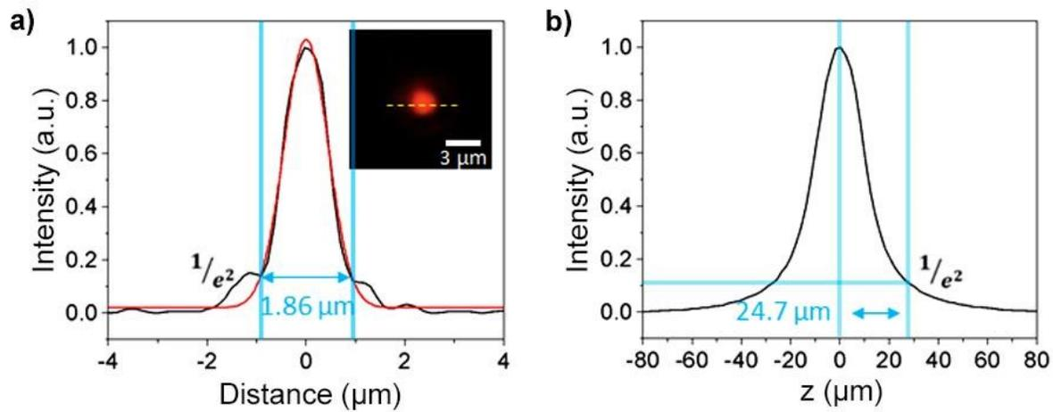
**Figure S1.** Laser beam (633 nm) profile and Raman intensity-depth profile based on the integrated intensity of the  $520.6 \text{ cm}^{-1}$  band for a silica wafer.
