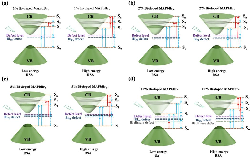
**Figure S6.** Four-level models of Bi-doped MAPbBr<sub>3</sub>/PMMA with different doping concentrations. (a) 1% Bi-doped; (b) 2% Bi-doped; (c) 5% Bi-doped; (d) 10% Bi-doped.
