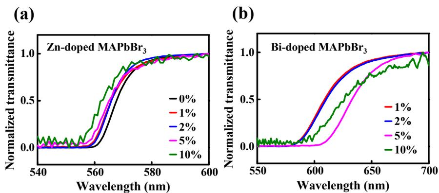
**Figure S1.** Transmission spectra of the undoped, Zn-doped and Bi-doped MAPbBr<sub>3</sub> with different doping concentrations.
