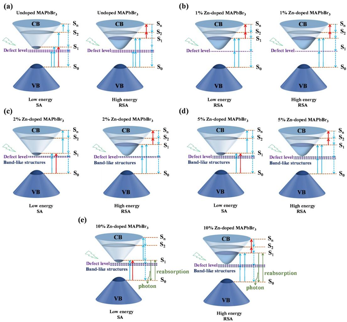
**Figure S4.** Four-level models of undoped and Zn-doped MAPbBr<sub>3</sub>/PMMA with different doping concentrations. (a) undoped ( 0% Zn-doped); (b) 1% Zn-doped; (c) 2% Zn-doped; (d) 5% Zn-doped; (e) 10% Zn-doped.
