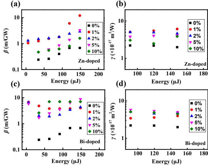
**Figure S5.** Dependence between  $\beta$  or  $\gamma$  and the incident pulse energy of undoped, Zn-doped and Bi-doped MAPbBr<sub>3</sub>/PMMA with different doping concentration.
