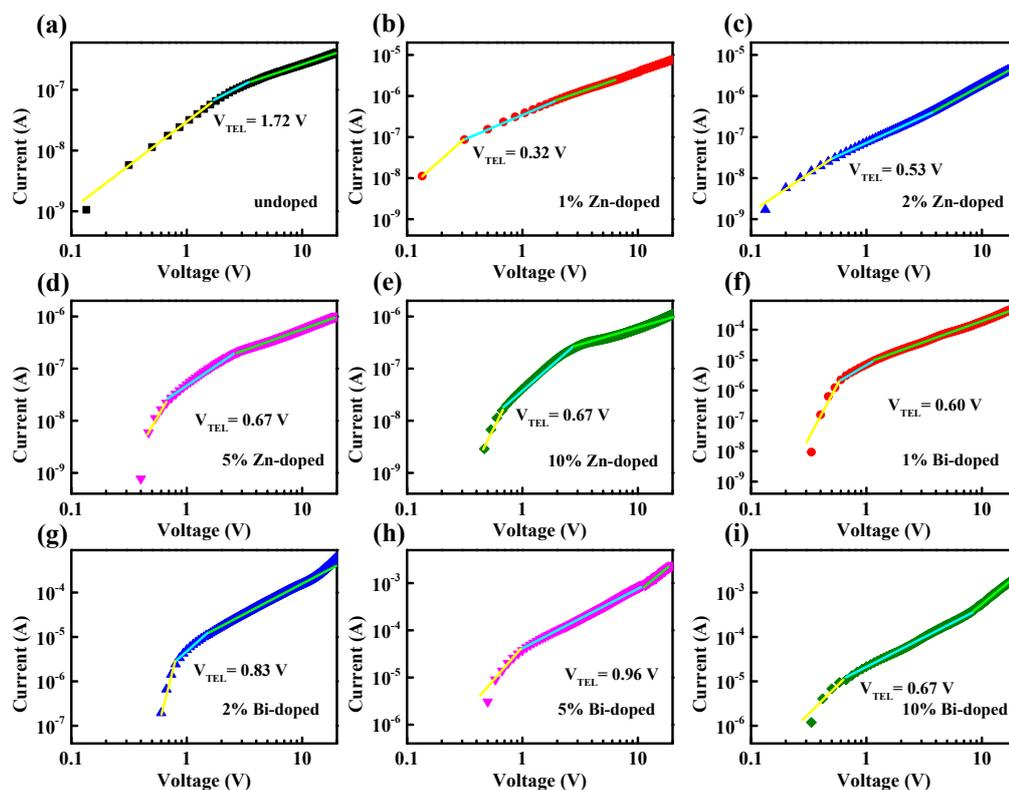
**Figure S2.** Double logarithmic current-voltage curves of the undoped, Zn-doped and Bi-doped MAPbBr<sub>3</sub>.
