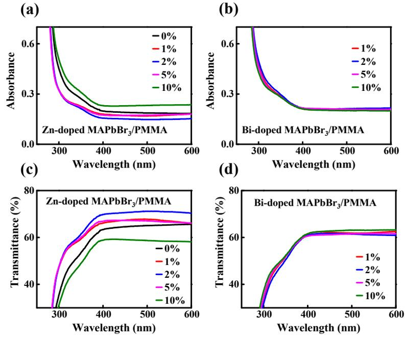
**Figure S3.** UV-vis absorption and transmission spectra of the undoped, Zn-doped and Bi-doped MAPbBr<sub>3</sub>/PMMA with different doping concentrations.
