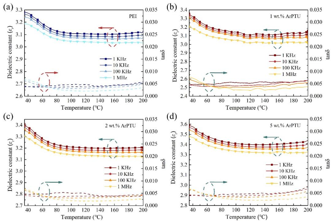
Figure S7. Temperature-dependent loss and dielectric constant of PEI and PEI/ArPTU composite films.
