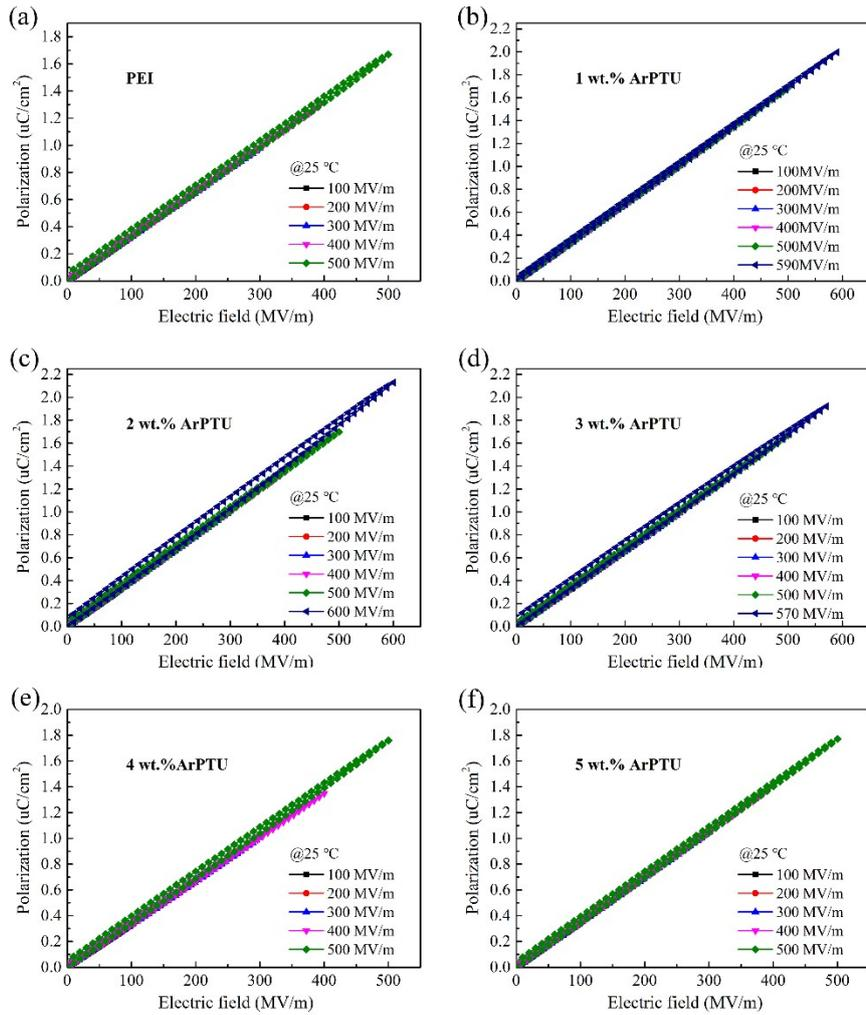
Figure S10. P-E loops of PEI/ArPTU composite films at 25 °C.
