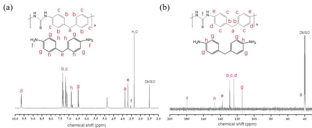
Figure S2. NMR spectra of ArPTU in DMSO-d<sub>6</sub>.
