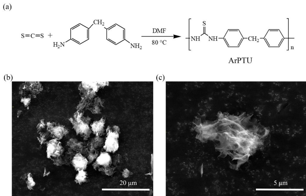
Figure S1. ArPTU synthesis equation and SEM images of ArPTU particles.
