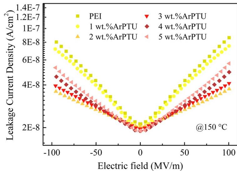
Figure S8. The leak current of ArPTU/PEI composite films at  $150^{\circ}\text{C}$ .
