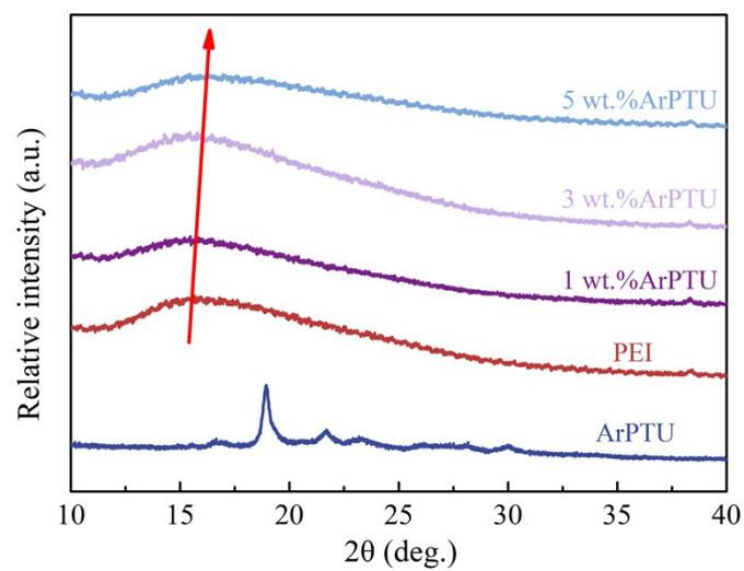
Figure S3. XRD patterns of composite films with different ArPTU contents.
