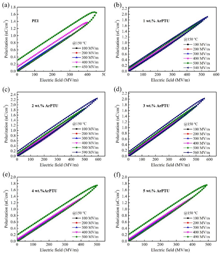
Figure S11. P-E loops of PEI/ArPTU composite films at 150 °C.
