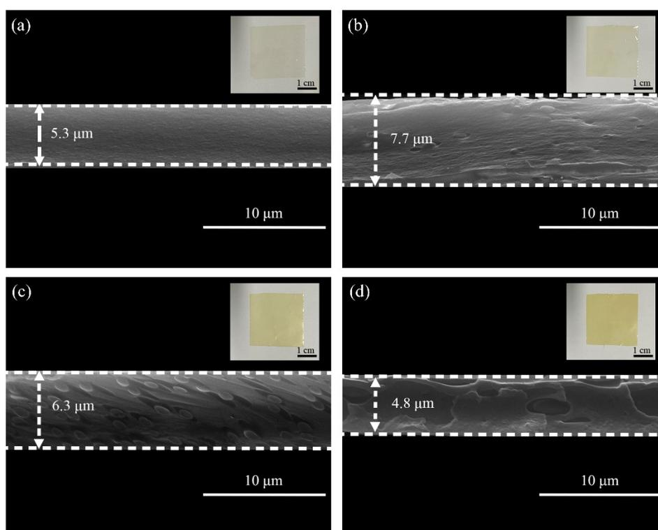
Figure S4. SEM images of PEI and 1 wt.%, 3 wt.%, 5 wt.% ArPTU composite films cross-section.
