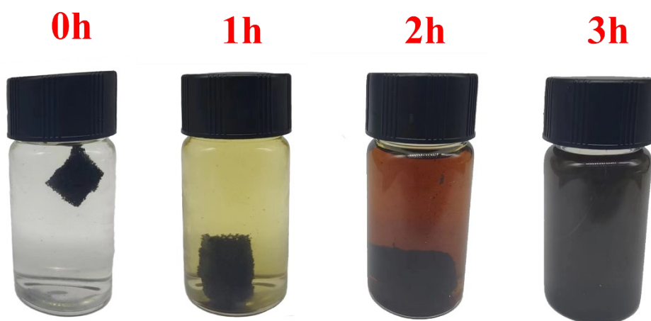
Figure S9: Digestion process of superhydrophobic, conductive LPUF in alkaline 0.5 mol/L NaOH methanolic solution at 60°C.
