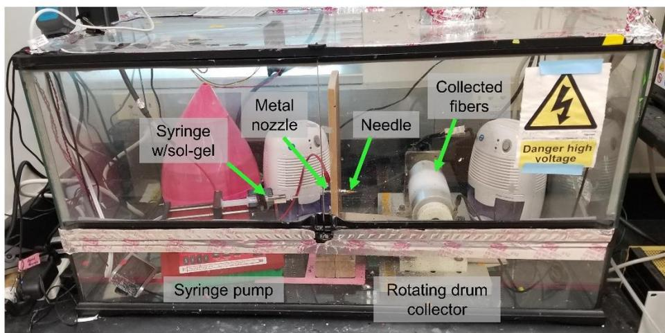
**Figure S3.** Photograph of the lab-scale, custom-built electrospinning enclosure used for nanofiber fabrication, with key components labeled.
