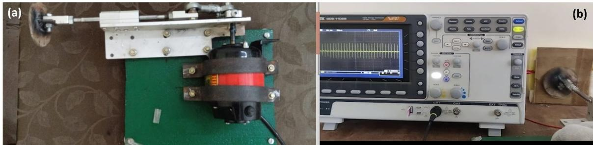
**Figure. S5.** Photographs of the (a) modified linear motor, (b)TENG response in DSO.
