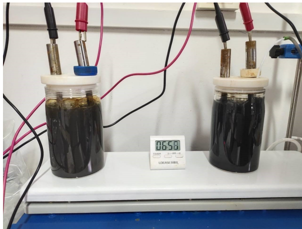
Fig. S1. Photo of the electrocoagulation experiment using scrap iron. The cylindrical cell is 128 mm of height and 78 mm of diameter.
