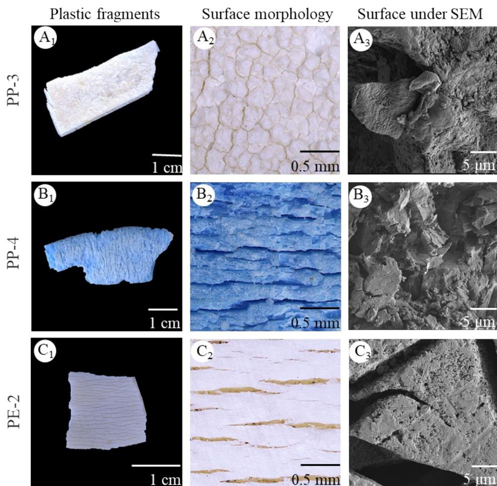
Fig. S2 Morphological characteristics of plastic pieces from the environments. A<sub>1</sub>-C<sub>1</sub> and A<sub>2</sub>-C<sub>2</sub> are obtained using optical microscope; A<sub>3</sub>-C<sub>3</sub> is obtained using SEM.
