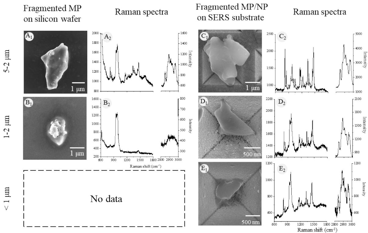
Fig. S4 SEM images and Raman spectra of MPs/NPs on the SERS substrate and silicon wafer
