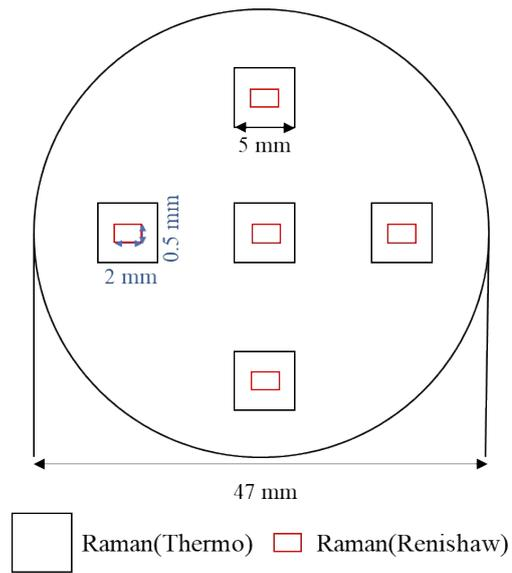
Fig. S1 Detected area using two different Raman. (Raman (Thermo Scientific™ DXR™ 3) with 20X magnification object and 785 nm laser was used to identify the large MPs (size > 50 μm); Raman (Renishaw, inVia Reflex, UK) with 50X magnification object and 785 nm laser was used to identify the small MPs (size of 10-50 μm))
