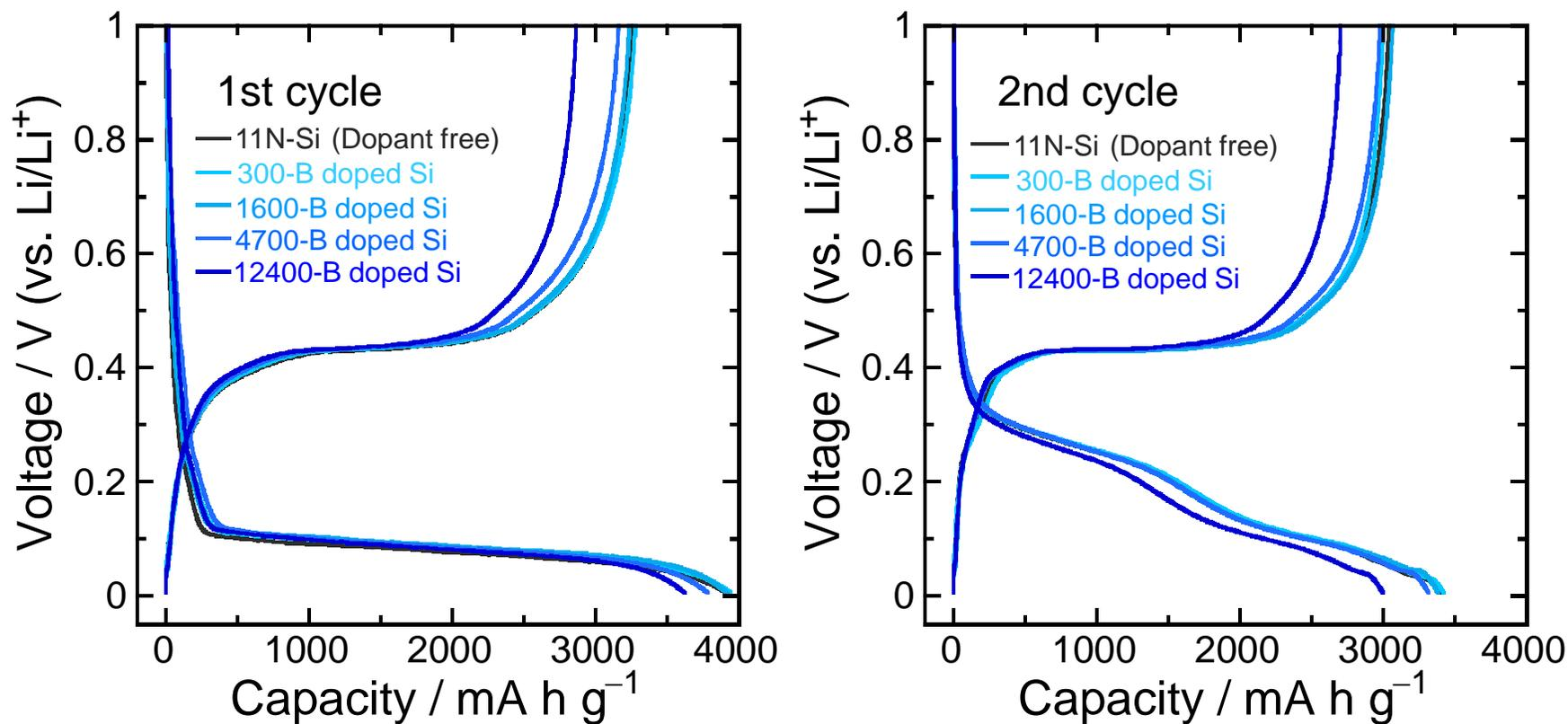
**Figure S4.** Comparison of first and second charge–discharge curves (Figure 2a) of undoped (dopant free) and B-doped Si (600, 1600, 4700, and 12400 ppm) electrodes in 1 M  $\text{LiPF}_6/\text{EC}:\text{DEC}$  (50:50 vol.%) at a current density of  $358 \text{ mA g}^{-1}$  ( $0.1C$ ). The onset voltages of lithiation for the B-doped Si are higher than that of the undoped Si irrespective of B concentrations.
