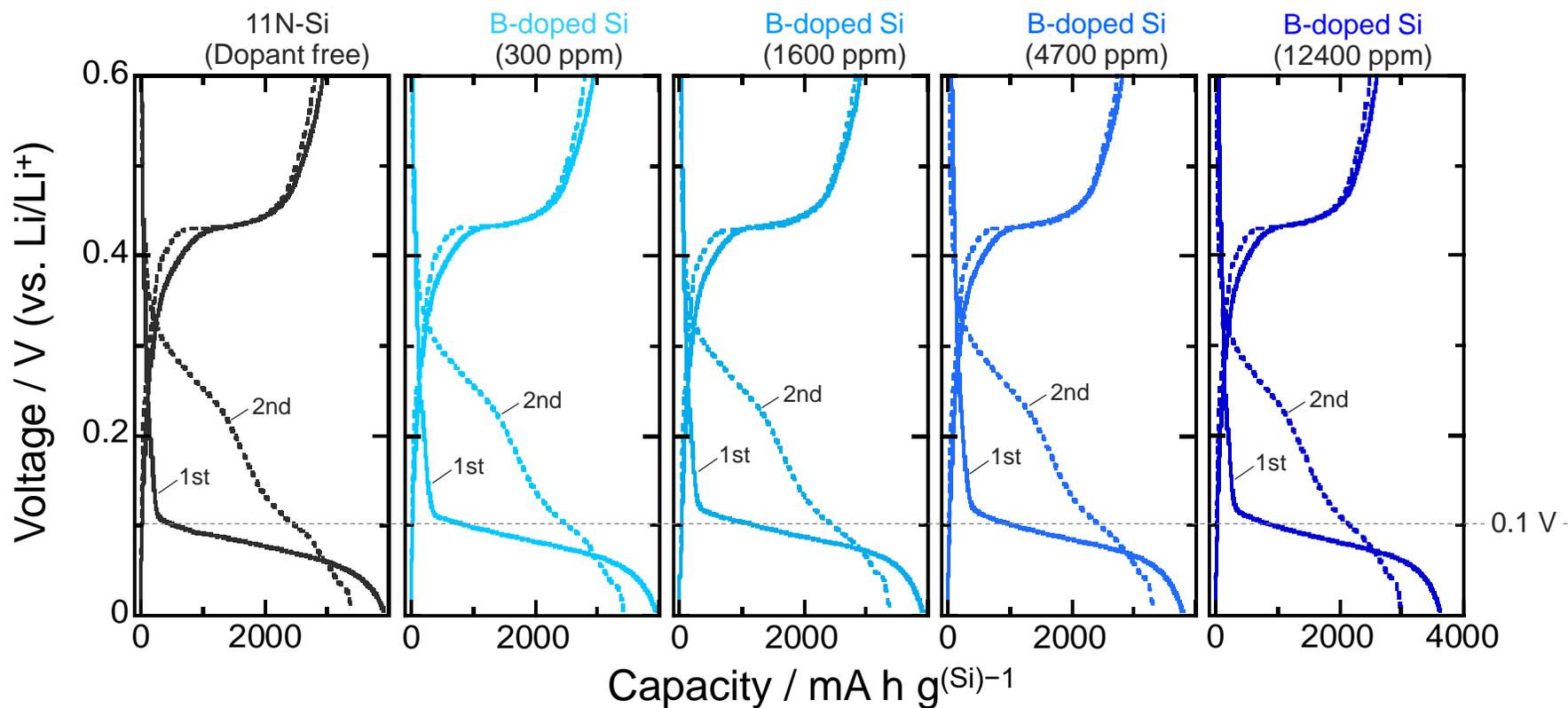
**Figure S3.** Enlarged view of galvanostatic charge–discharge curves (Figure 2a) of undoped (dopant free) and B-doped Si (600, 1600, 4700, and 12400 ppm) electrodes in 1 M  $\text{LiPF}_6/\text{EC}:\text{DEC}$  (50:50 vol.%) at a current density of  $358 \text{ mA g}^{-1}$  ( $0.1C$ ). The onset voltages of lithiation for the B-doped Si are higher than that of the undoped Si irrespective of B concentrations.
