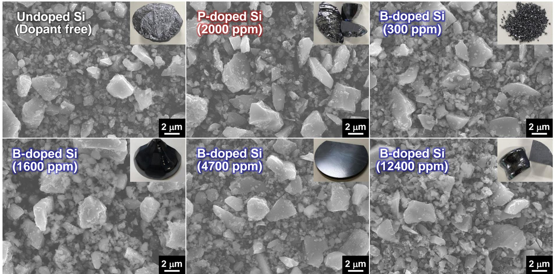
**Figure S1.** SEM images of 11N-Si (dopant free), P-doped Si (2000 ppm), B-doped Si (600, 1600, 4700, 12400 ppm) powders crushed by mechanical milling. Insets: Si ingots prepared by the Czochralski method (300 ppm-B doped Si: crushed granules). the 300 ppm-B doped Si was prepared from a diluted melt of the Si with highly concentrated B and polycrystalline Si.
