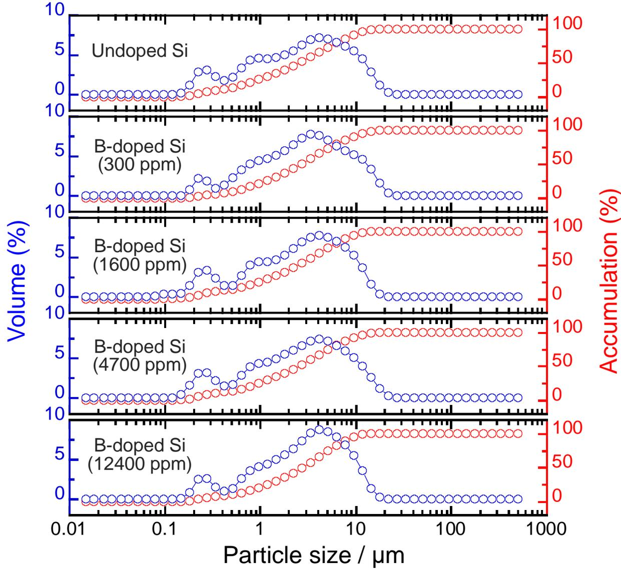
**Figure S2.** Particle size distributions of 11N-Si (dopant free) and B-doped Si (600, 1600, 4700, 12400 ppm) powders used in the preparation of mixture electrodes in this work. Ingots were fractured to granule size in a mortar prior to mechanical milling (MM). The respective MM times were set to keep the particle size distributions about the same.
