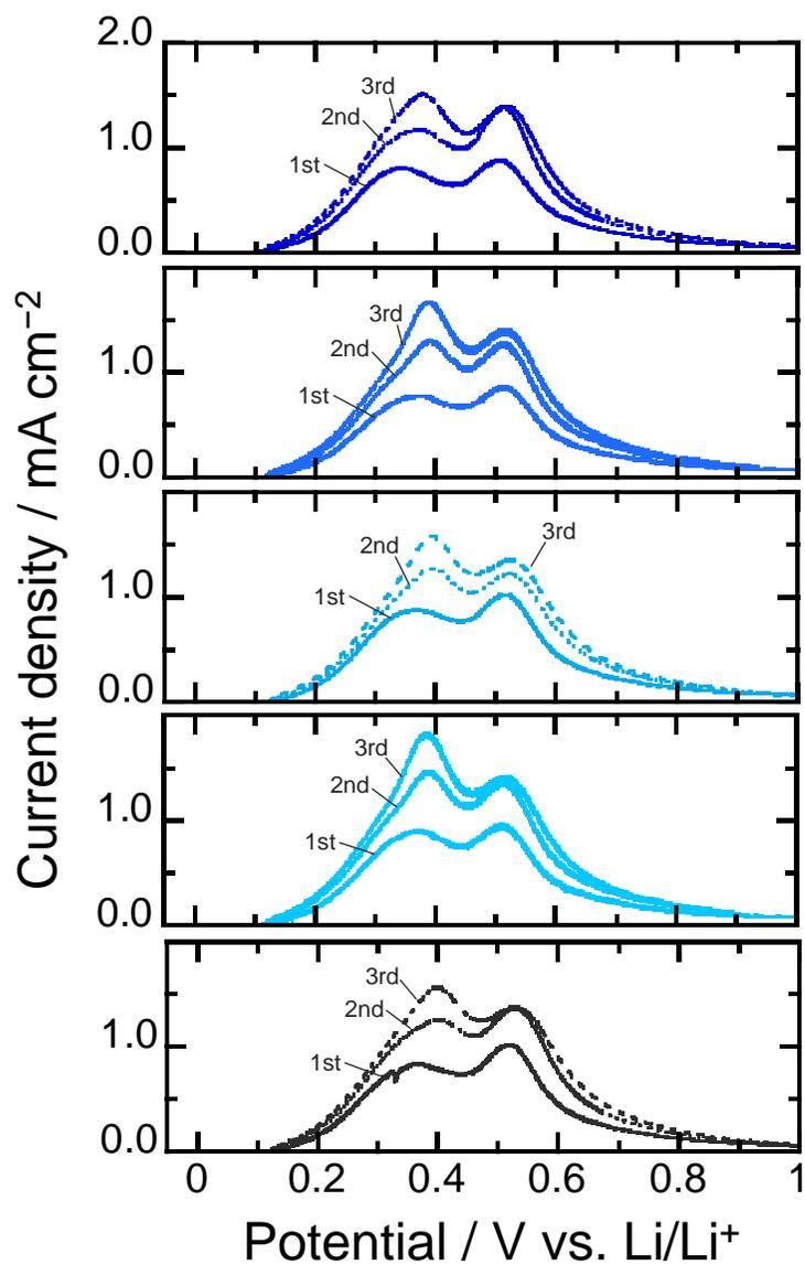
**Figure S6.** Cyclic voltammograms of undoped and B-doped Si (600, 1600, 4700, and 12400 ppm) electrodes in 1 M LiPF<sub>6</sub>/EC:DEC (50:50 vol.%) at a sweep rate of 0.1 mV s<sup>-1</sup>. Left: cathodic scan, Right: anodic scan.
