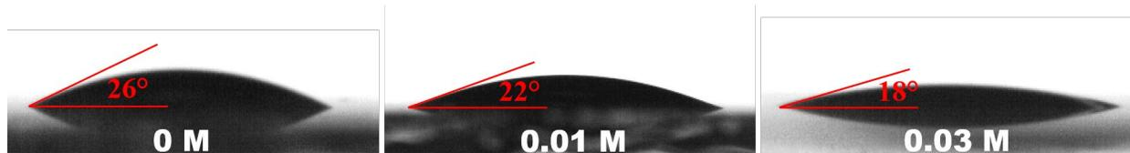
*Figure S8. Water contact angle of the  $\text{TiO}_2$  surface with [TMPA][TFSI] modification.*
