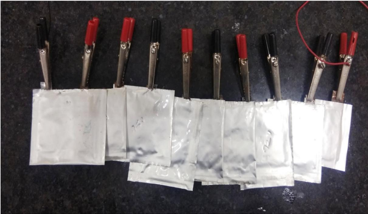
**Fig. S5** assemble the 10 pouch cells of 1.2V and 890 mAh in series connection. All specific sizes can be clearly seen through these optical images, which directly affect the storage and charge exchange mechanism.
