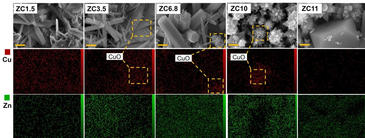
Figure S3. FESEM images and the corresponding distribution of Cu and Zn elements carried out with EDS mapping of the samples (the scale bar shows 1  $\mu\text{m}$ )
