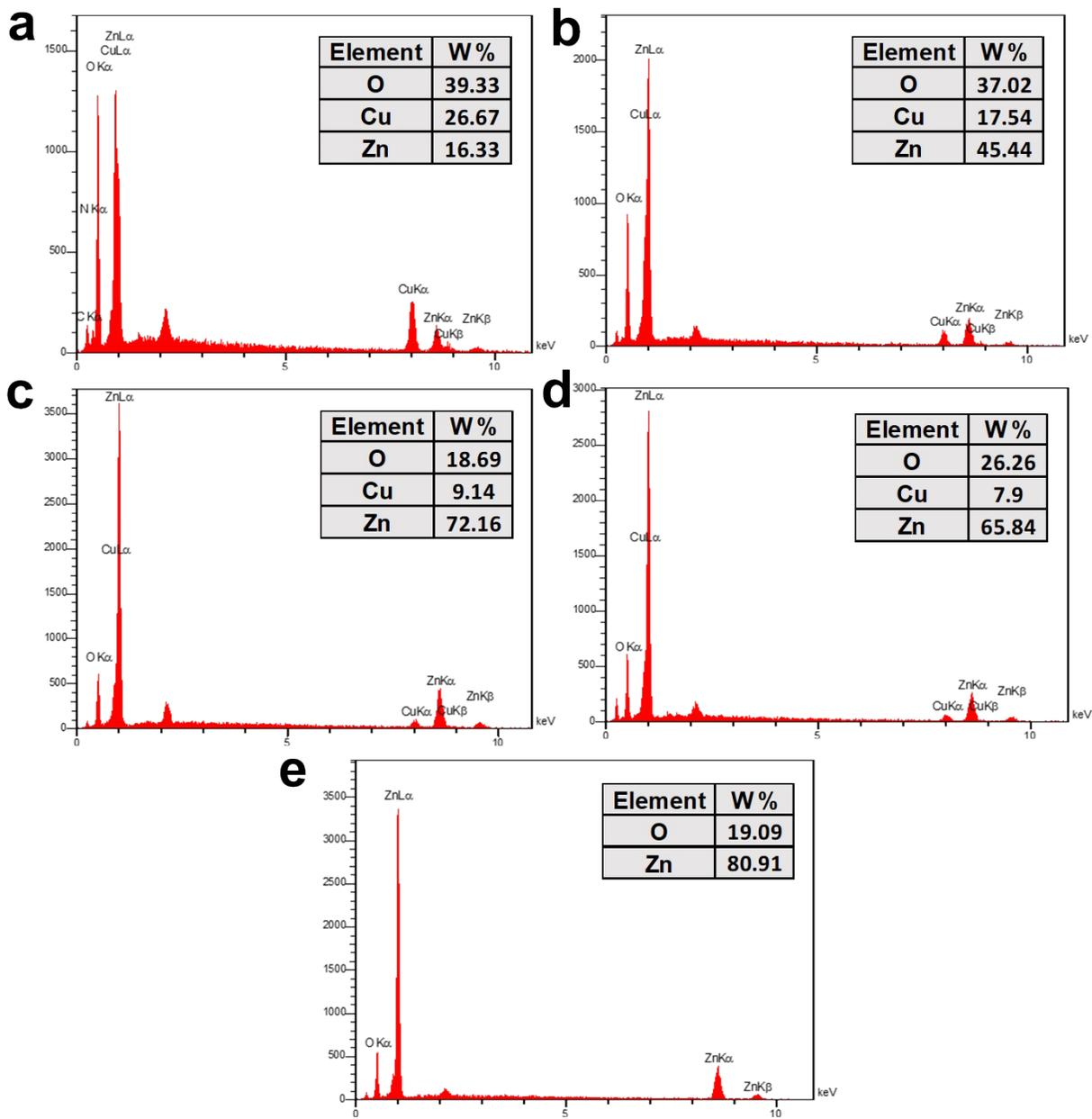
Figure S2. EDS analysis of samples (a) ZC1.5, (b) ZC3.5, (c) ZC6.8, (d) ZC10, (e) ZC11 illustrating the quantitative content of O, Cu, and Zn elements.
