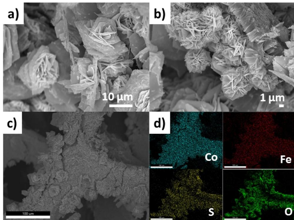
Figure S7 a-c) FESEM micrographs of S-CoFeLDH/NF after electrochemical stability. d) elemental mapping corresponding to Co, Fe, S and O.
