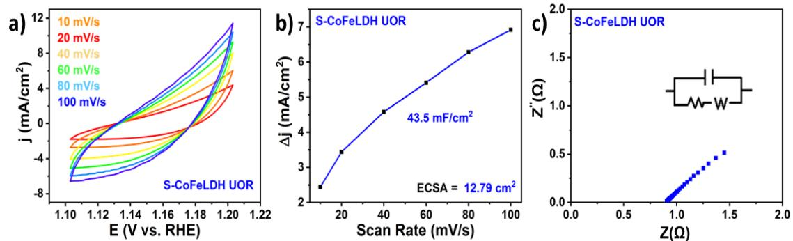
Figure S6 Electrochemical measurements for UOR a) CV at different scan rates, b) Cdl plot and c) EIS nyquist plot of S-CoFeLDH in 1 M KOH with 0.5 M Urea
