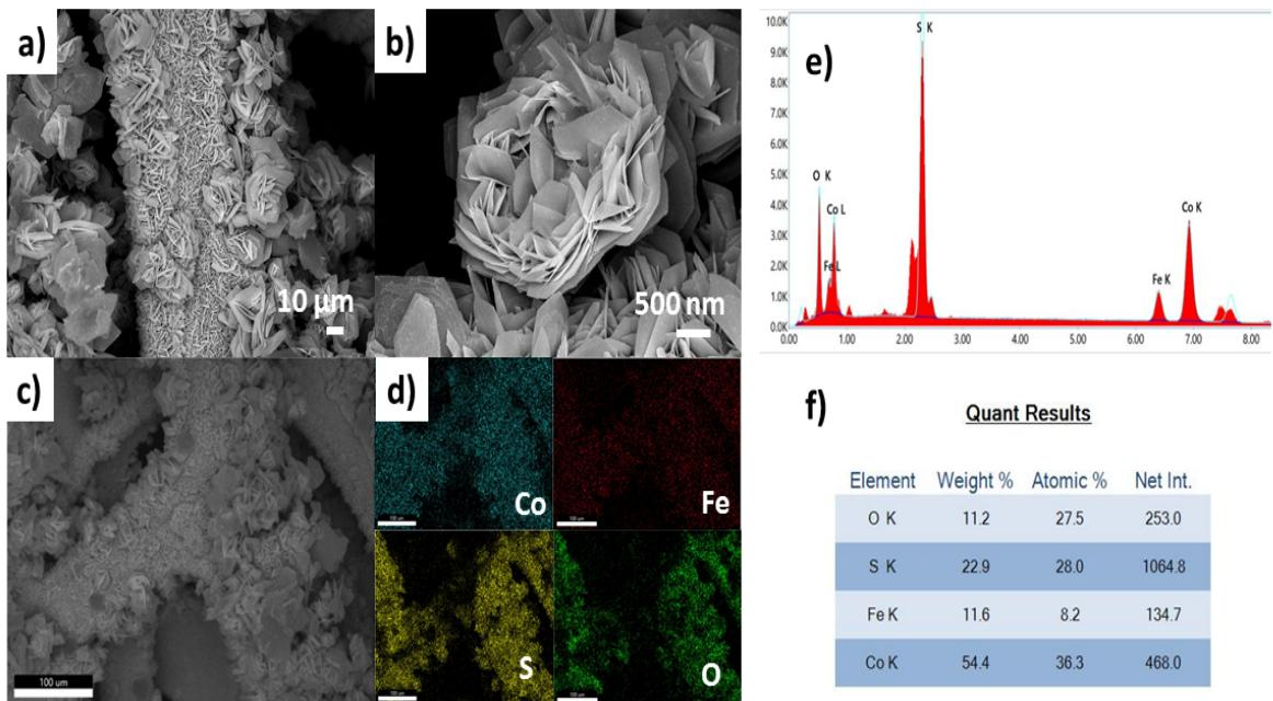
Figure S3 a-c) FESEM micrographs of S-CoFeLDH at different resolutions. d) Corresponding elemental mapping of Co, Fe, S and O. e-f) EDAX and corresponding quantitative results of elements
