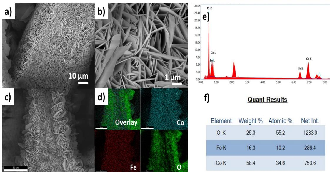
Figure S2a-c) FESEM micrographs of CoFeLDH/NF at different resolution. d) Corresponding elemental mapping of Co, Fe and O. e) EDAX f) Quantitative Results of elements
