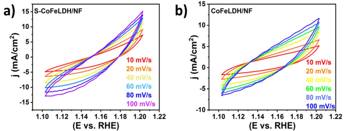
Figure S4 CV voltammogram of a) S-CoFeLDH/NF and b) CoFeLDH/NF
