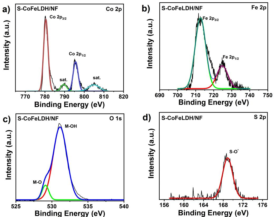
Figure S8 XPS analysis after electrochemical stability. High resolution XPS of a) Co2p b) Fe2p c) O1s and d) S2p
