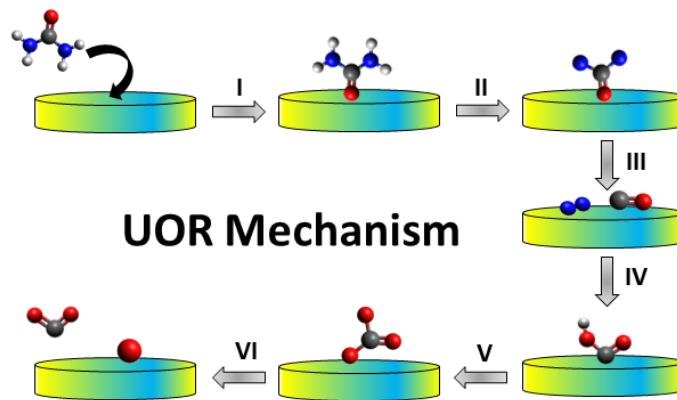
Figure S10: Detailed UOR mechanism.
