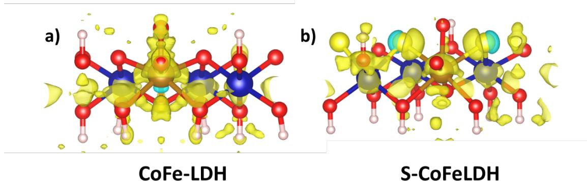
Figure S12: Differential charge density curve a) CoFe-LDH and b) S-CoFeLDH.
