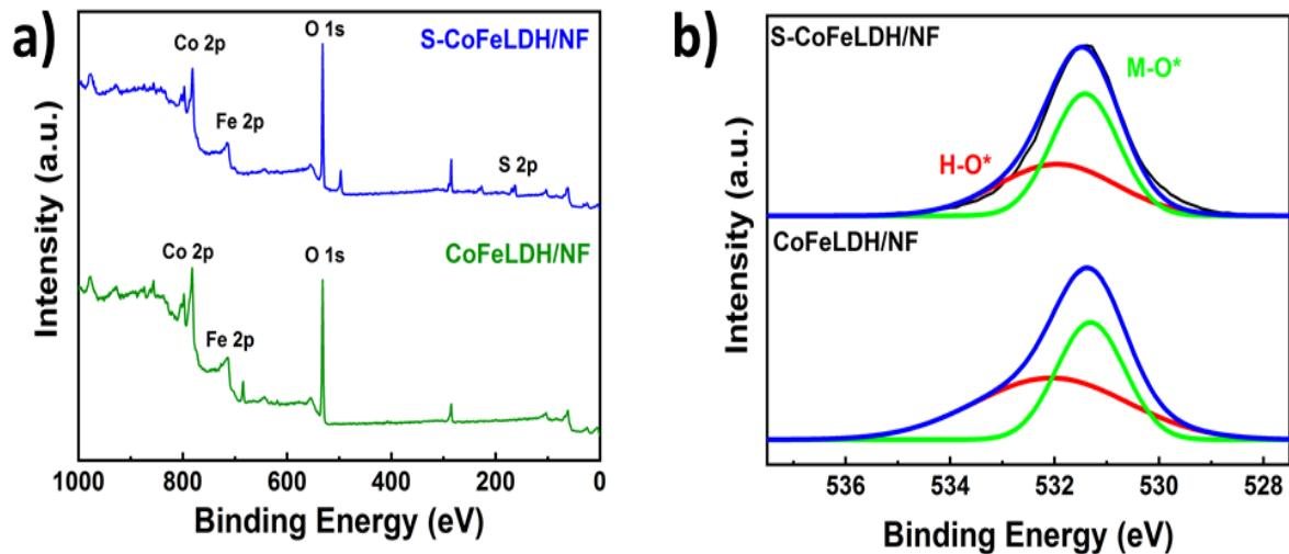
Figure S1 a) Wide scan survey spectrum of S-CoFeLDH/NF b) High resolution XPS of O 1s in S-CoFeLDH/NF
