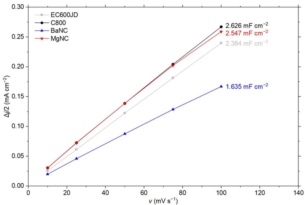
**Fig. S2.** Dependences between scan rate and supercapacitive current for carbon electrodes in nitrogen-saturated phosphate buffer solution (pH = 6.0).
