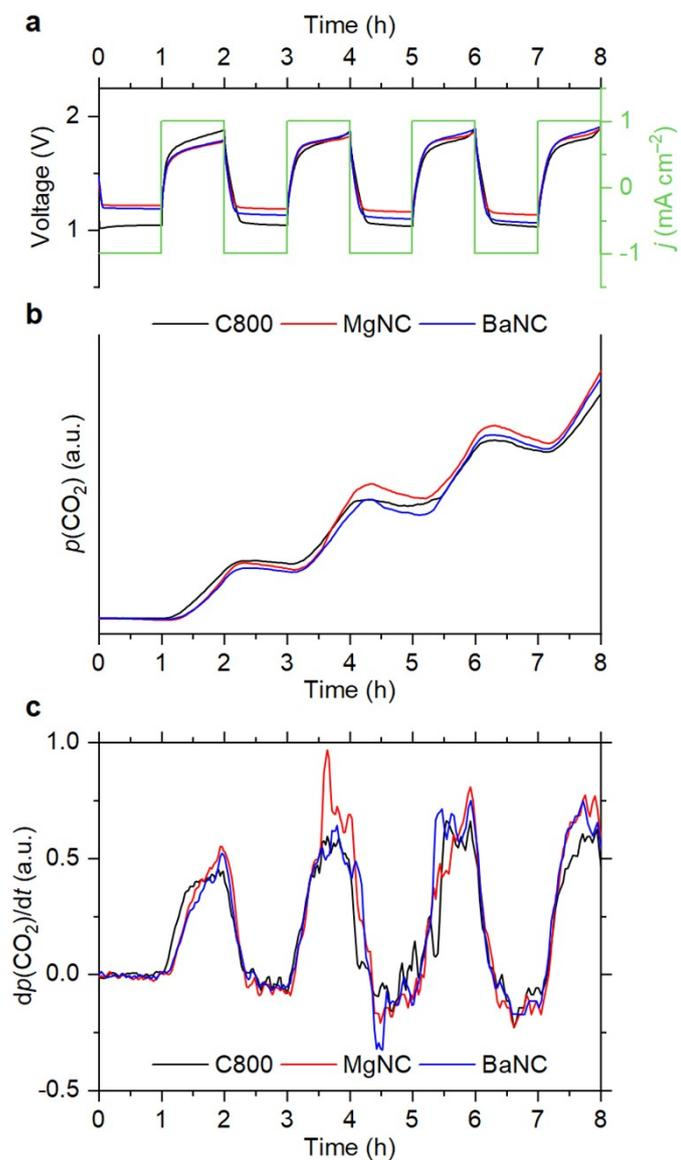
**Fig. S6.** Zn-air cell voltage and current density vs. time (a), evolution of CO<sub>2</sub> partial pressure (b) and its derivative (c) during the OEMS measurements.
