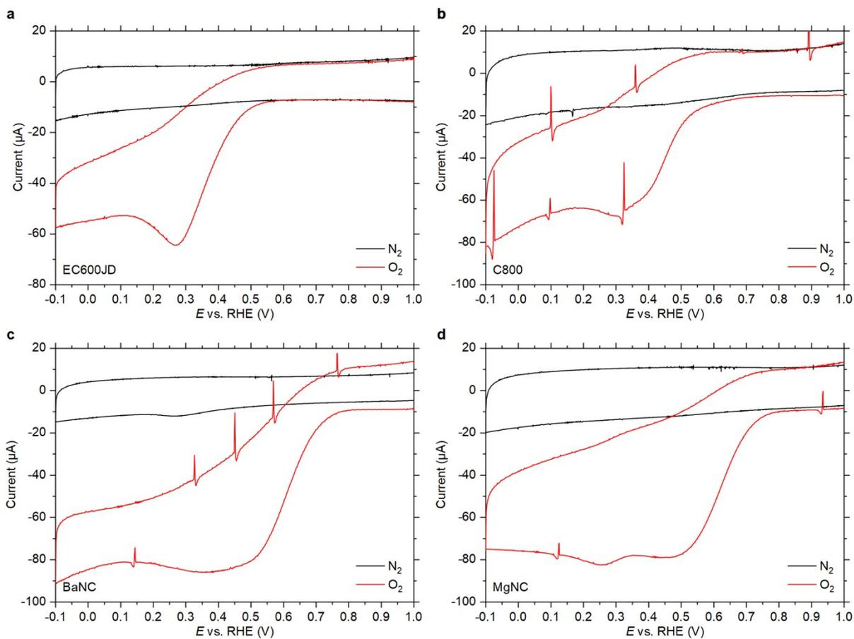
**Fig. S1.** CV response of EC600JD (a), C800 (b), BaNC (c) and MgNC (d) in nitrogen- and oxygen-saturated phosphate buffer solution (pH = 6.0).
