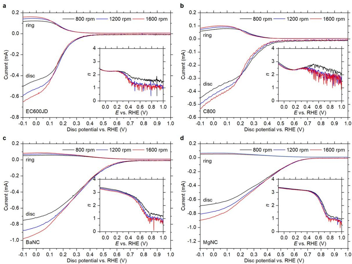
**Fig. S4.** Ring/disk currents and electron transfer numbers (insets) for EC600JD (a), C800 (b), BaNC (c) and MgNC (d) electrodes, measured in RRDE experiments with oxygen-saturated phosphate buffer solution (pH = 6.0).
