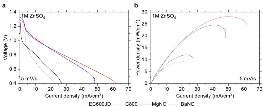
**Fig. S5.** Current-voltage (a) and current-power (b) plots for Zn-air cells with various cathode materials during an LSV scan ( $10 \text{ mV s}^{-1}$ ) with 1M ZnSO<sub>4</sub> electrolyte.
