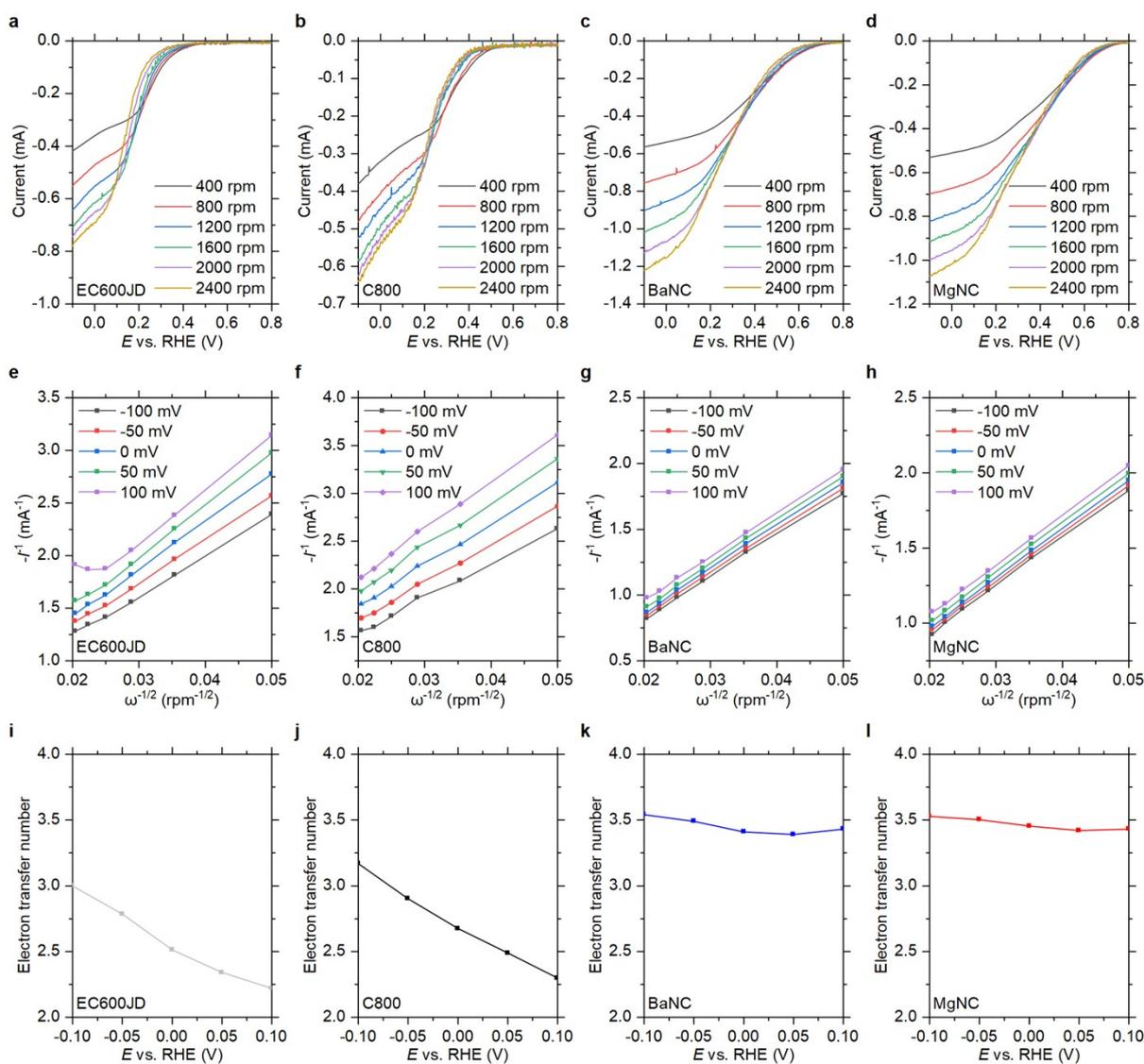
**Fig. S3.** RDE experiments (a-d), corresponding Koutecky–Levich plots for various potentials vs. RHE (e-h) and estimated electron transfer numbers (i-l) for EC600JD (a, e, i), C800 (b, f, j), BaNC (c, g, k) and MgNC (d, h, l), measured in oxygen-saturated phosphate buffer solution (pH = 6.0).
