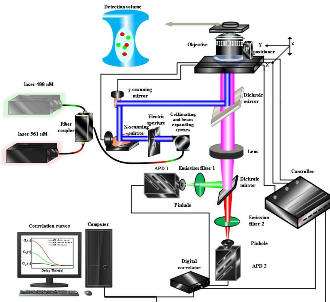
Fig. S9 The setup of the San-FCS/San-FCCS system.
