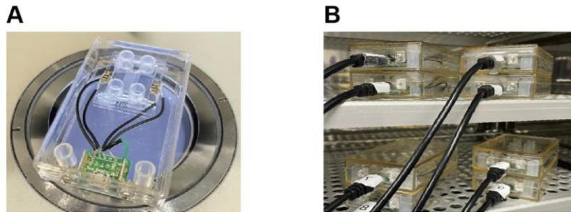
Supplementary Figure 1. Photographs of our MPS and TEER measurement setup. A. The devices were mounted on a polystyrene case and were connected to LCR meters USB connectors, allowing measurements inside an incubator. B. Simultaneous measurements of up to 8 devices made from multiple devices inside the incubator by connecting the cable from the outside via a custom-made unit of relay circuits.
