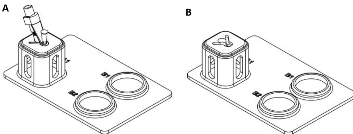
Figure S2: Technical drawings of the writing head holder with (A) and without (B) the writing head. This piece protects the writing head from damage when it is not attached to the robot's pipette. Before archiving, the robot picks up the writing head from its
