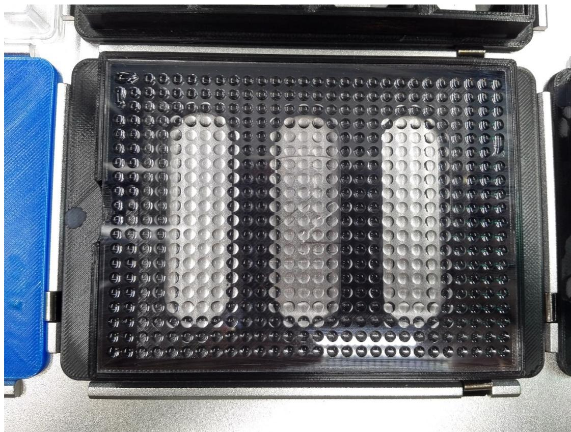
*Figure S4: An overhead view of the SET after archiving. Some isolated incidents of cross talk between neighbouring SETs can be observed. These incidents are limited to the left and right edges of the SET array, as well as the upper left corner, where the separation begins. These locations are where the writing head is changing direction and thus unable to maintain a smooth,*
