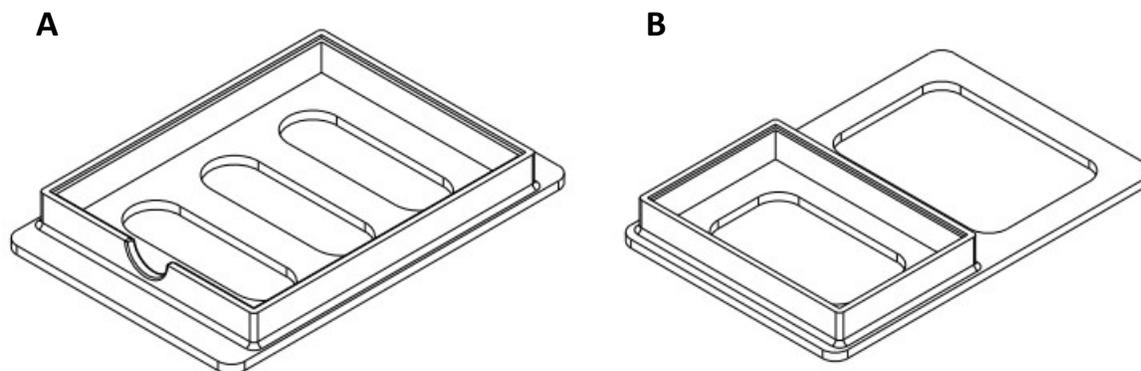
Figure S1: Technical drawings of the slide holders used to mount the SET arrays to the bed of the OT-2 pipetting robot. The 4"x3" slide holder is pictured in A, while the 50mmx75mm (2"x3") slide holder is pictured in B. The footprint of each slide holder matches a standard 96 well plate.
