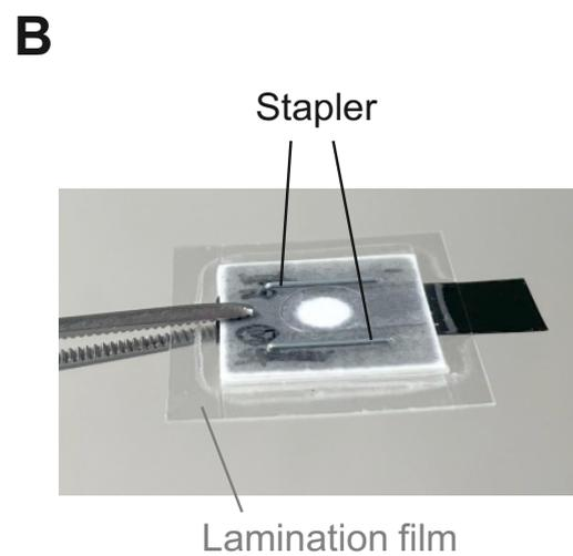
**Fig. S5** (A) Illustration of the sandwich structure consisting of three paper-layers, time adjustment film, and double-sided tape. (B) Photograph of the fully integrated device.
