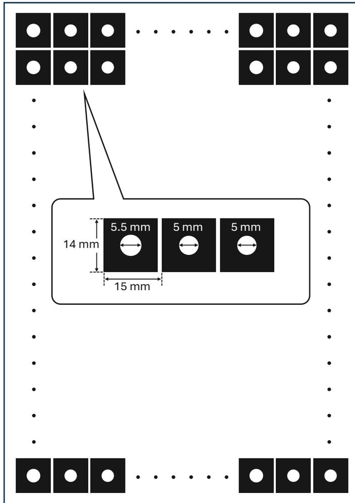
**Fig. S2** The wax printing pattern designed using Adobe Illustrator CC software. Black areas were printed using the wax-printer.
