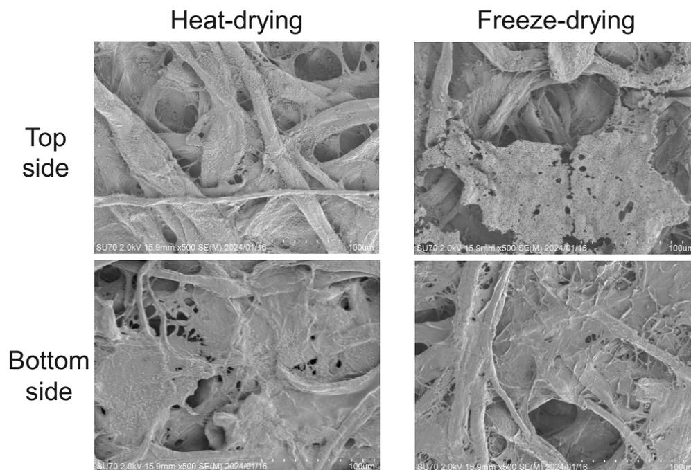
**Fig. S7** SEM images of the top and bottom sides of paper substrates (A5C) on which MB conjugates and Cas12a-crRNA complex have been (left) heat-dried or (right) freeze-dried. The presence of MB conjugates was confirmed on both sides of the paper substrate in the case of heat-drying, while they were observed only on the top side when freeze-dried.
