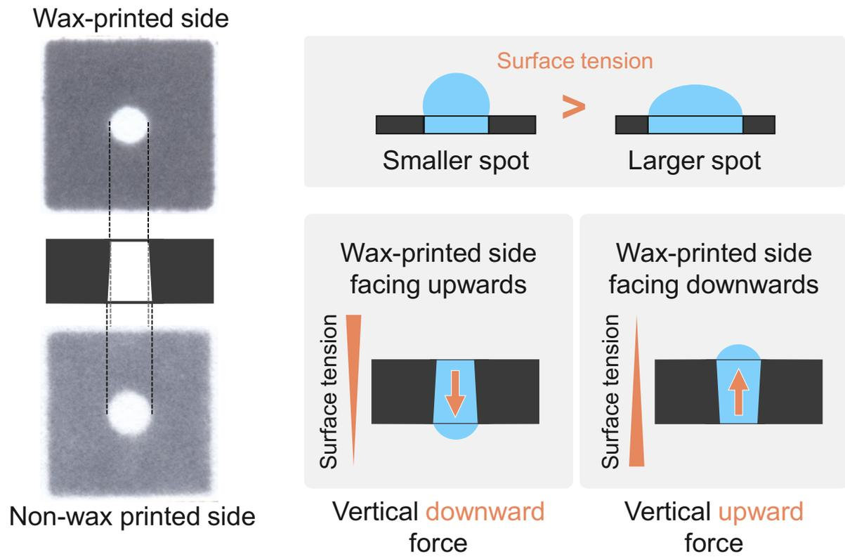
**Fig. S10** Schematic of the dependence of wax-printed paper orientation on vertical sample flow caused by the conical frustum shape of a wax-patterned circular spot.
