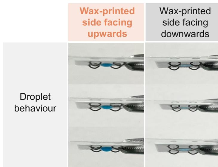
**Fig. S9** Dependence of liquid dye droplet formation on orientation of wax-printed paper side in a fully integrated multilayer paper device: (A) wax-printed side facing upwards and (B) wax-printed side facing downwards.
