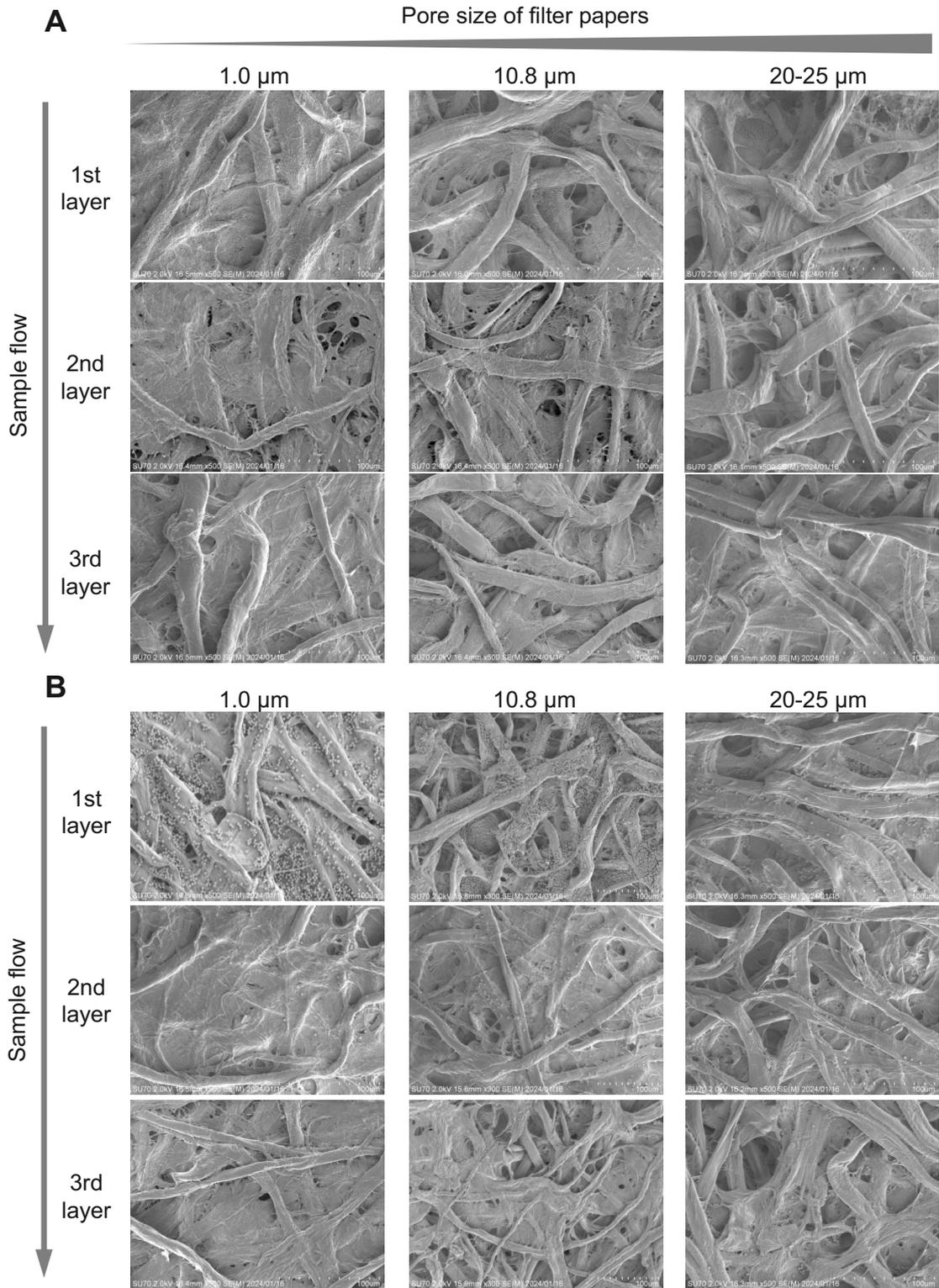
**Fig. S6** SEM images of the front side of each paper layer after assays without adding sucrose solution with using different pore size of filter papers and (A) 1.0 and (B) 2.8  $\mu\text{m}$  of MBs. It can be confirmed that the number of MBs on 2<sup>nd</sup> and 3<sup>rd</sup> layer is decreased as MBs size increases and pore size of filter papers decreases, suggesting successful filtration of MBs by filter papers.
