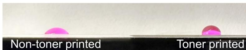
**Fig. S3** Comparison of water droplet behaviour on non-toner modified transparency film (left) and toner printed film (right). The picture indicates a larger contact angle for the toner-modified film, proving the successful hydrophobic treatment of the transparency film by toner printing.
