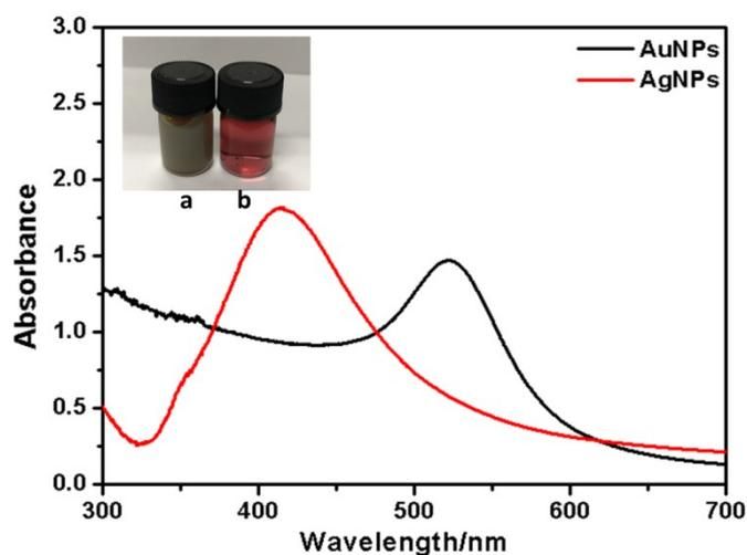
Fig.S1 The absorption spectra of (a) silver nanoparticles colloid (b) gold nanoparticles colloid.
