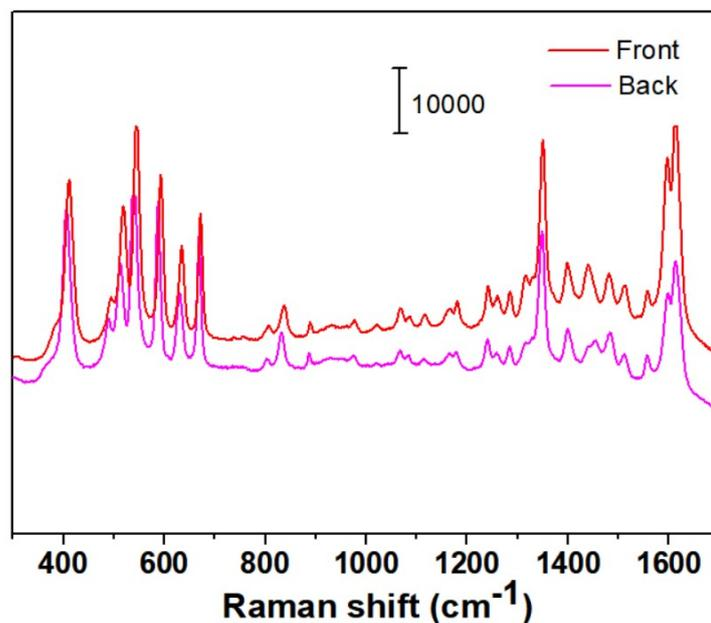
Fig.S3 the SERS spectra of pyocyanine at the concentration of  $10^{-4}$ M collected from the front and back on the Nano-silver SERS substrate
