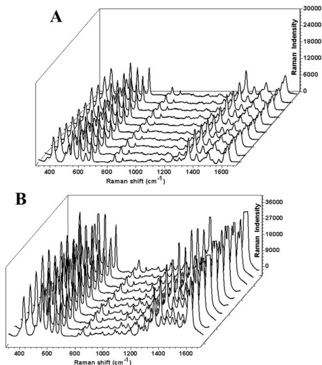
Fig. S4 The collected SERS spectra of pyocyanin on (a) gold SERS substrate and (b) silver SERS substrate at 10 randomly spots.
