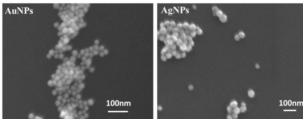
Fig.S2 Morphology characterization of silver and gold nanoparticles by SEM
