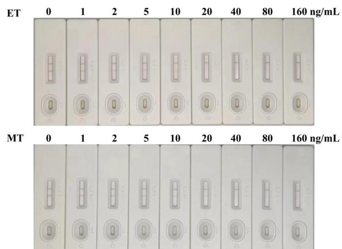
**Fig. S3.** The test images of GNP-LFIA for the determination of ET and MT spiked in water.
