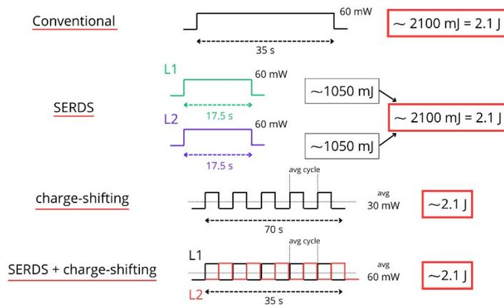
Figure S2. Schematics of the laser intensity and acquisition time for the investigated methods.
