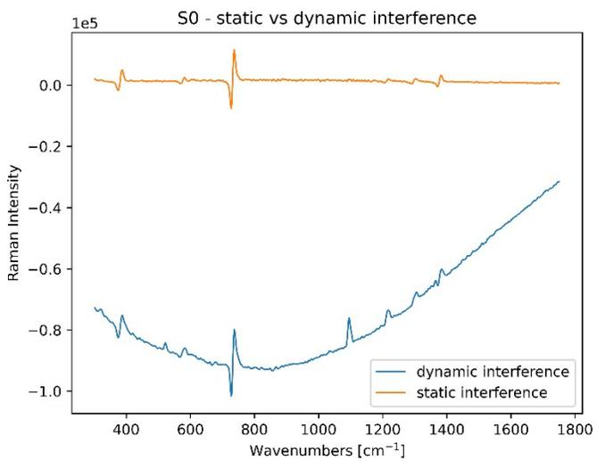
Figure S5. Comparison of SERDS measurements of S0 with static or dynamic background interference. It is clear that in the latter case even SERDS struggles to provide an appreciable result.
