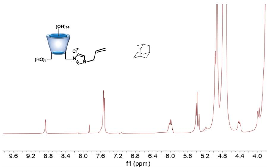
**Fig. S-14.**  $^1\text{H}$  NMR spectra of the AICD mixed with adamantane were obtained after a dissolution period of 24 h in  $\text{CD}_3\text{OD}/\text{D}_2\text{O}$  (40/60, v/v).
