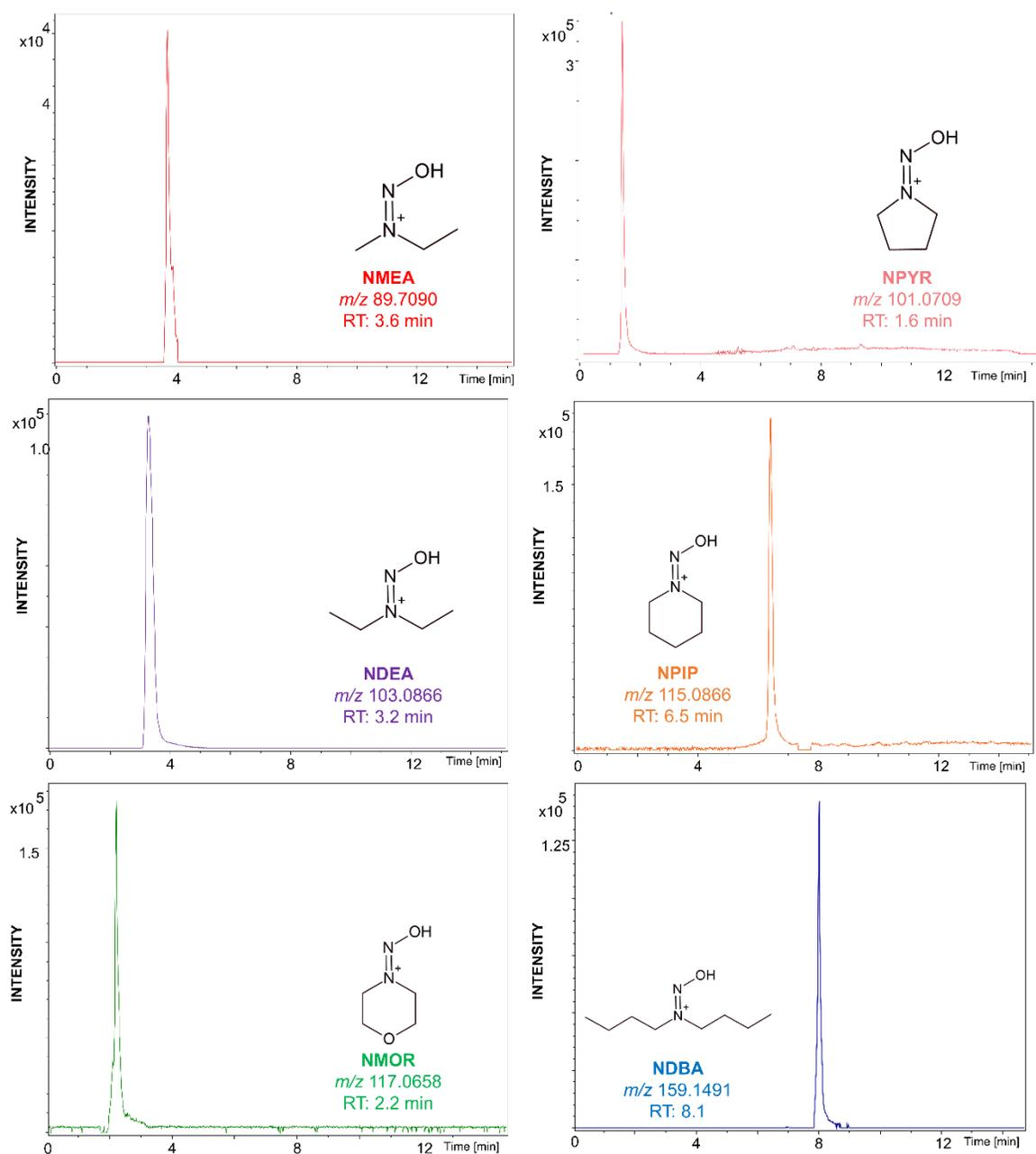
**RT:** Retention time; **NMEA:** N-nitroso-N-methylethylamine; **NPYR:** N-nitrosopyrrolidine; **NDEA:** N-nitrosodiethylamine; **NPIP:** N-nitrosopiperidine; **NMOR:** N-nitrosomorpholine; **NDBA:** N-nitroso-N-dibutylamine.
