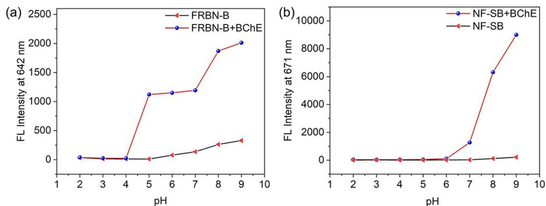
**Fig. S3.** Fluorescence intensity curve of (a) **FRBN-B** (10  $\mu\text{M}$ ,  $\lambda_{\text{ex}} = 579 \text{ nm}$ ; Slit: 5 nm/5 nm) and (b) **NF-SB** (10  $\mu\text{M}$ ,  $\lambda_{\text{ex}} = 579 \text{ nm}$ ; Slit: 10 nm/10 nm) in different pH values of HEPES buffer solution in the presence and absence of BChE (0.5 U/mL).
