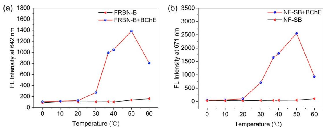
**Fig. S4.** Fluorescence intensity curve of (a) **FRBN-B** (10  $\mu\text{M}$ ,  $\lambda_{\text{ex}} = 579 \text{ nm}$ ; Slit: 5 nm/5 nm) and (b) **NF-SB** (10  $\mu\text{M}$ ,  $\lambda_{\text{ex}} = 579 \text{ nm}$ ; Slit: 10 nm/10 nm) at different temperatures in the presence and absence of BChE (0.5 U/mL).
