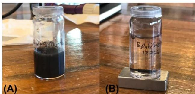
**Figure Sa:** A) Fe<sub>3</sub>O<sub>4</sub>@SiO<sub>2</sub>-APTES @Au NPs dispersed in an aqueous solution and (B) after magnetic separation.
