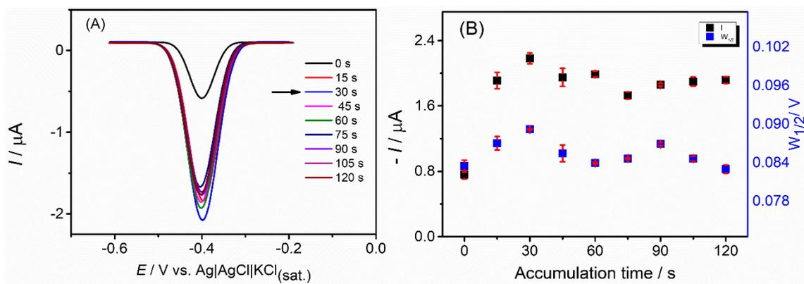
**Figure S3.** (A) Baseline-corrected DPV responses recorded for  $50 \mu\text{mol L}^{-1}$  of CAP in  $0.12 \text{ mol L}^{-1}$  BR buffer as function of accumulation time. (B) Peak currents (black squares) and peak width half height (blue squares) as function of accumulation time. Conditions: Step potential,  $5 \text{ mV}$ ; modulation amplitude,  $60 \text{ mV}$ ; modulation time,  $50 \text{ ms}$ ; interval time,  $0.5 \text{ s}$ .
