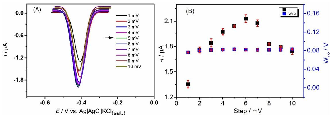
**Figure S4.** (A) Baseline-corrected DPV voltammograms obtained for  $50 \mu\text{mol L}^{-1}$  of CAP in  $0.12 \text{ mol L}^{-1}$  BR buffer as function of step potential. (B) Peak currents (black squares) and peak width half height (blue squares) as function of step potential. Conditions: accumulation time,  $30 \text{ s}$ ; modulation amplitude,  $60 \text{ mV}$ ; modulation time,  $50 \text{ ms}$  and interval time,  $0.5 \text{ s}$ .
