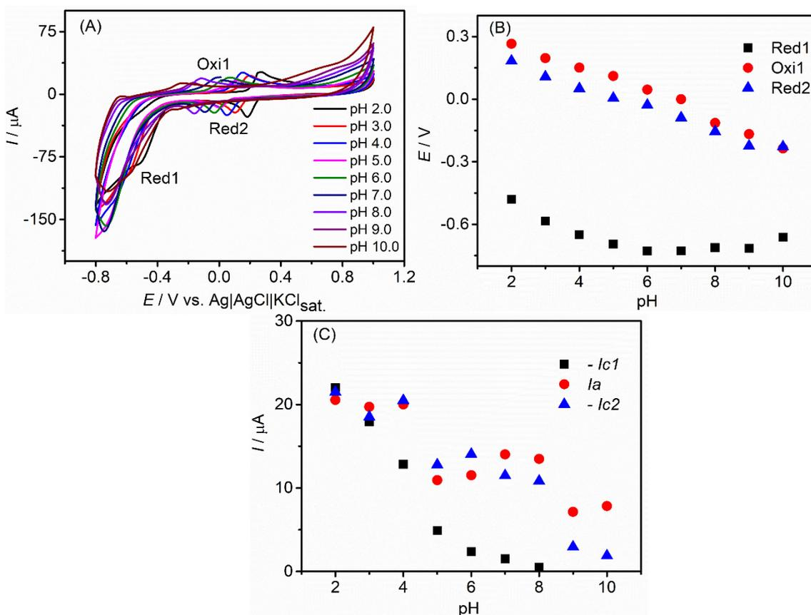
**Figure S1.** (A) Cyclic voltammetric recordings for CAP (0.5 mmol L<sup>-1</sup>) in 0.12 mol L<sup>-1</sup> BR buffer solution (pH range from 2.0 to 10.0). (B) pH influence at peak potential ( $E_p$ ) and (C) pH influence at peak current ( $I_p$ ). Conditions: step potential, 5 mV scan rate, 50 mV s<sup>-1</sup>.
