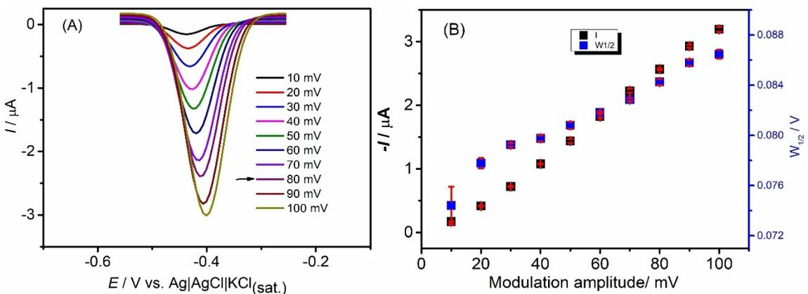
**Figure S5.** (A) Baseline- corrected DPV responses recorded for  $50 \mu\text{mol L}^{-1}$  of CAP in  $0.12 \text{ mol L}^{-1}$  BR buffer as function of modulation amplitude. (B) Peak currents (black squares) and peak width half height (blue squares) as function of modulation amplitude. Conditions: accumulation time, 30 s; step potential, 5 mV; modulation time, 50 ms s and interval time, 0.5 s.
