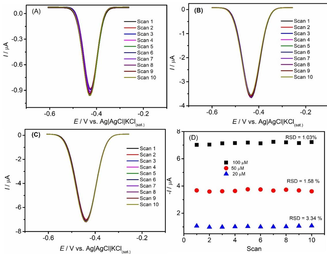
**Figure S7.** Repeatability data obtained from successive scan ( $n = 10$ ) for CAP solution containing: (A) 20; (B) 50 and (C)  $100 \mu mol L^{-1}$ . Conditions: Table S1.
