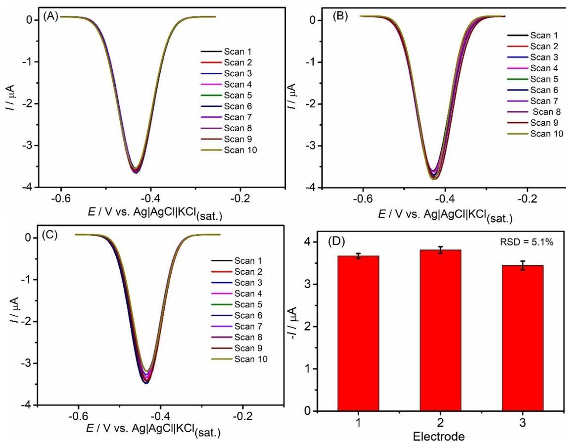
**Figure S8.** Reproducibility data obtained from successive scan ( $n = 10$ ) for CAP solution containing  $50 \mu\text{mol L}^{-1}$  at three different electrodes. Conditions: table S1.
