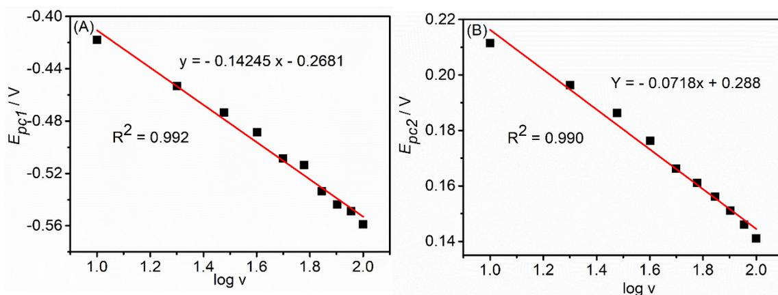
**Figure S2.** (A and B) Relationship between peak potential ( $E_p$ ) and  $\log v$ .
