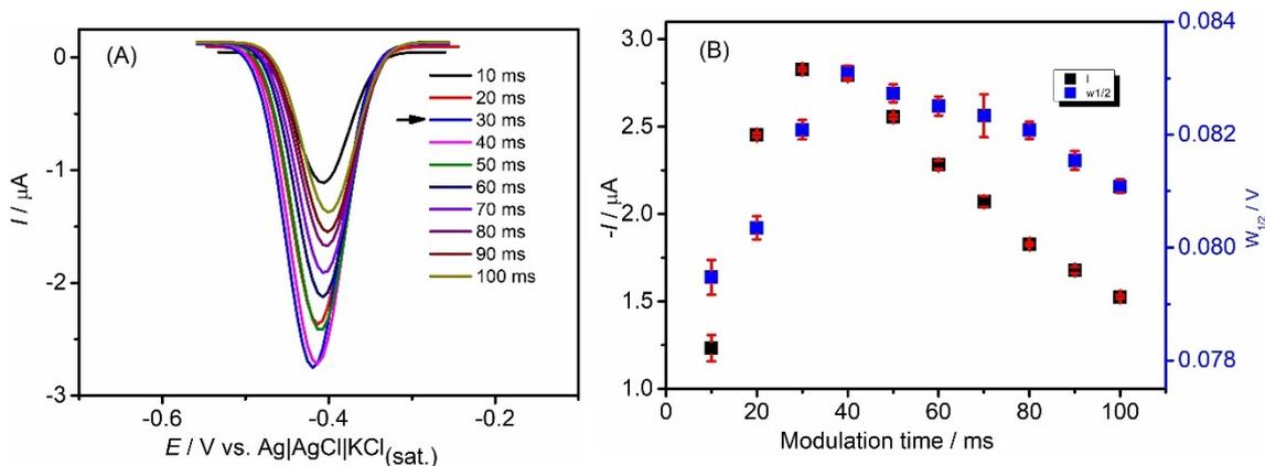
**Figure S6.** (A) DPV (corrected baseline) measures for  $50 \mu\text{mol L}^{-1}$  of CAP in  $0.12 \text{ mol L}^{-1}$  BR buffer as function of modulation time. (B) Peak currents (black squares) and peak width half height (blue squares) as function of modulation time. Conditions: accumulation time, 30 s; step potential, 5 mV; modulation amplitude, 80 mV s and interval time, 0.5 s.
