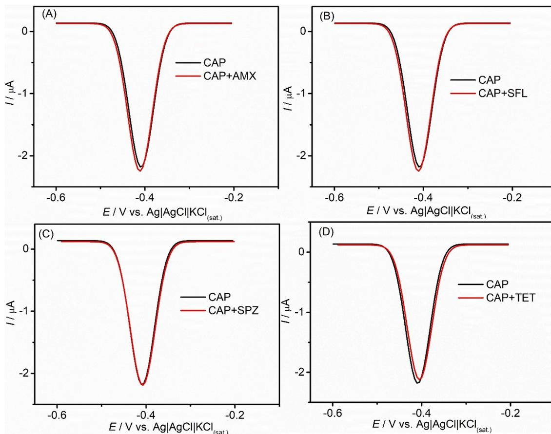
**Figure S9.** Baseline-corrected DPV voltammograms obtained for CAP  $50 \mu\text{mol L}^{-1}$  and the equimolar mixture ( $50 \mu\text{mol L}^{-1}$ ) of CAP and interferents (A) AMX; (B) SFL; (C) SFZ and (D) TET under optimized instrumental conditions.
