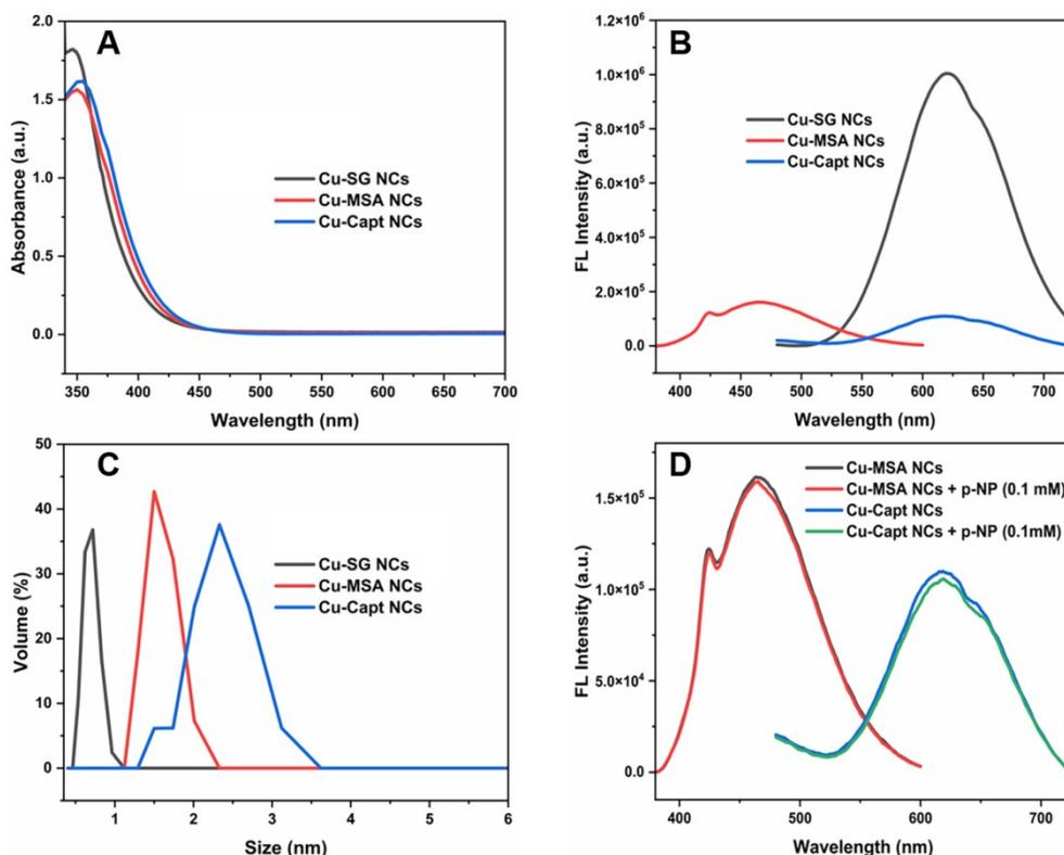
**Fig. S7.** (A) The UV-vis absorption spectra of Cu-SG NCs, Cu-MSA NCs, and Cu-Capt NCs. (B) The luminescence spectra of Cu-SG NCs, Cu-MSA NCs, and Cu-Capt NCs. (C) The DLS of Cu-SG NCs, Cu-MSA NCs, and Cu-Capt NCs. (D) The luminescence of Cu-MSA NCs and its mixture with p-NP (0.1 mM), and Cu-Capt NCs and its mixture with p-NP (0.1 mM).
