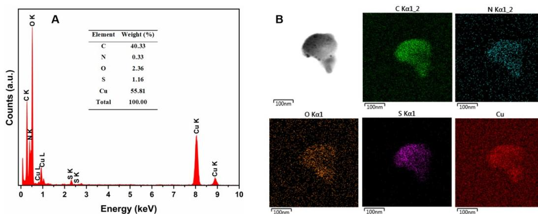
**Fig. S4.** (A) EDS spectra of Cu-SG NCs. (B) EDS elemental mapping images of C, N, O, S, and Cu for Cu-SG NCs.
