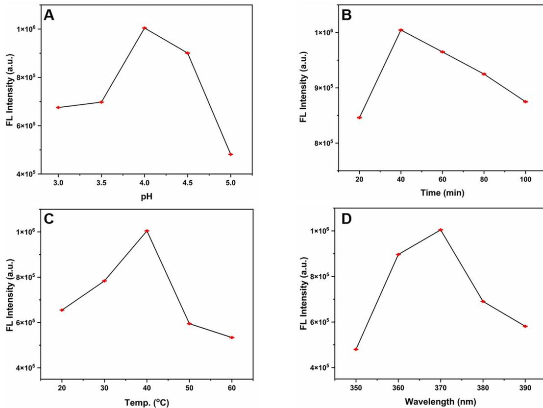
**Fig. S1.** The one-factor-at-a-time tests on fluorescence intensity dependencies on pH value (A), reaction time (B), temperature (C), and optimal excitation wavelength (D) for Cu-SG NCs.
