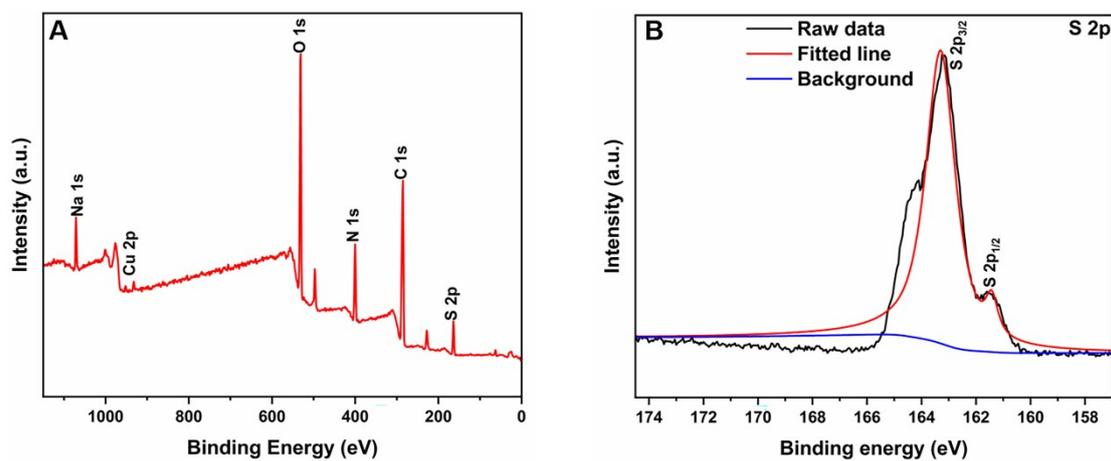
**Fig. S5.** (A) XPS spectra of the Cu-SG NCs. (B) High resolution XPS spectra of S2p.
