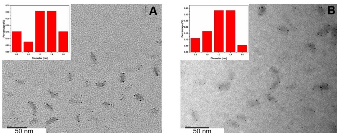
**Fig. S3.** (A) HRTEM images of Cu-SG NCs (inset: size distribution histogram). (B) HRTEM images of Cu-SG NCs with p-NP (0.5 mM) (inset: size distribution histogram).
