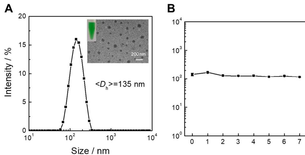
**Fig. S18** (A) Hydrodynamic diameter distribution profile of IR775-Cbl@PF127 in aqueous solution. The insets are TEM image and the photograph of IR775-Cbl@PF127 aqueous dispersion. (B) Hydrodynamic diameters recorded for the aqueous dispersion of IR775-Cbl@PF127 upon storage at room temperature.
